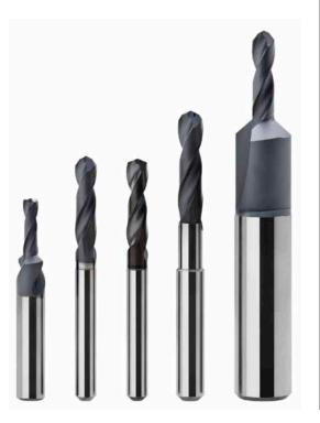
To combat the abrasive properties of carbon fiber reinforced polymer, the Feedmax –C1 and –C2 incorporate a polycrystalline diamond coating, which also provides good dimensional tolerance. The drills are 5xD with diameters ranging from 0.1260" – 0.5". All –C1 and –C2 drills also feature through-coolant holes.
