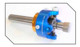
broaching brake to be used as an attachment to its innovative GT Series rotary broach holder. The brake mounts to the tool holder using set screws. Additional screws are included at the opening of the brake to gently tighten against the spindle. The broach is fastened into the spindle, and must make contact and be aligned at the first hole.
