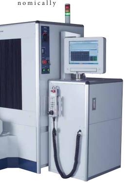
positioned touch-panel monitor with built-in compact keyboard, plus a builtin, industrial-grade controller and PC. It all means the MACH-3A CMM offers the functionality, durability and stability required for 24/7 in-line operation.
