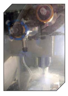
The rotary broaching brake is a lightweight, low-profile tool and easily fits into the VMC's tool changer. It easily slides onto the head of the holder and does not require special tools for adjustment or assembly. The brake can also be easily removed for operations where it is not required.
