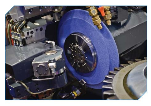
giving engineers a broad range of benefits in gear grinding, including increased throughput, less wheel dressing, a dramatically lower risk of burning, extended wheel life and consistent grinding performance.
