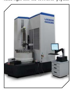
GAMA suite of applications' software. The new 1500GMS can also perform increasingly important Barkhausen noise testing to detect grind burn as just another routine step taken during the course of normal gear inspection. The 1500GMS uses proven Stresstech Rollscan 300 Analyzer technology integrated into the platform to save the time and setups usually required to perform Barkhausen off-line on other equipment,
