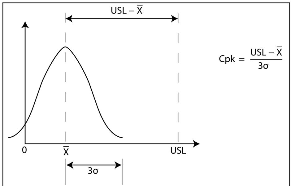
Figure 2 Cpk determination for a unilateral tolerance.
