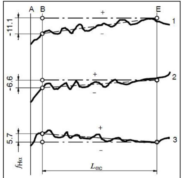
Figure 4 Average and Slope Variation — AGMA 915-1: average =  $(5.7 + (-6.6) + (-11.1)) / 3 = -4.6\mu\text{m}$ ; variation =  $5.7 - (-11.1) = 16.8\mu\text{m}$ .
