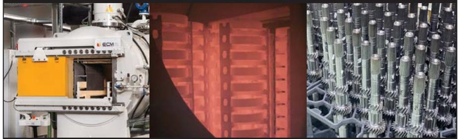
Low Pressure Vacuum Carburizing • Neutral Hardening • Oil Quenching
