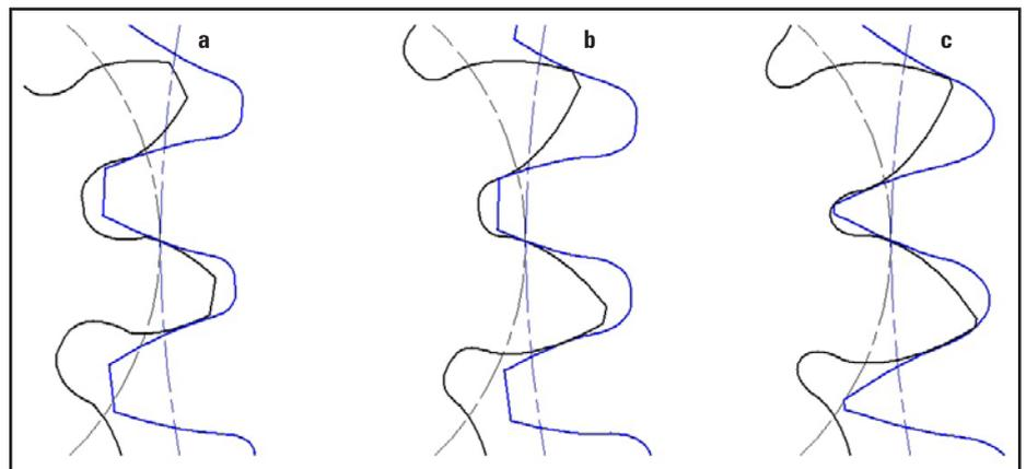
**Figure 1** Gear meshes of 10 and 40 tooth gears; a—standard (pressure angle 20°, X-shifts 0 and 0, contact ratio 1.08), b—standard (pressure angle 20°, X-shifts +0.5 and -0.5, contact ratio 1.40), c—nonstandard (pressure angle 22.5°, contact ratio 1.70)
