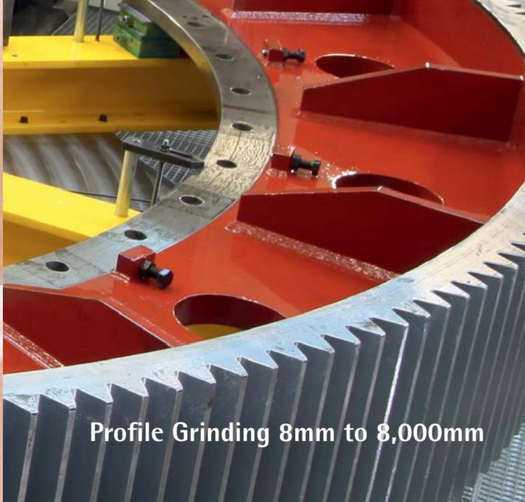
Profile Grinding 8mm to 8,000mm
