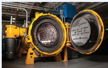
From stress relief to case hardening, our precise carbon control and aerospace qualified pyrometry produce uncompromised quality. Harness our leading-edge vacuum technology to improve the uniformity of your case depths, minimize distortion and enjoy clean parts with no IGO (intergranular oxidation).
