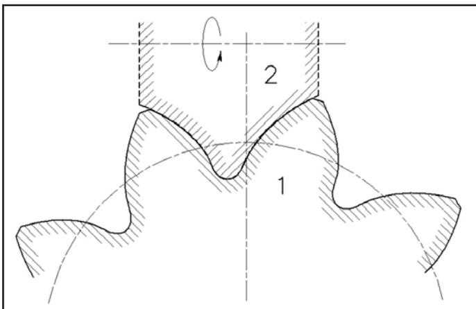
Figure 1 Gear form machining: 1) gear profile; 2) tool profile.
