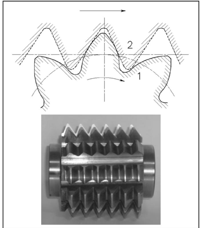
Figure 4 a. rack generating: 1) gear profile; 2) hob or rack cutter profile; b. asymmetric gear hob cutter.
