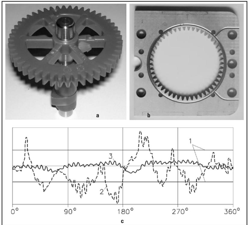
**Figure 11** Genetic Molding Solution application: a) camshaft gear; b) gear mold cavity; c) roll rest chart overlay; 1) total composite tolerance limits; 2) initial specimen chart; 3) final gear chart.
