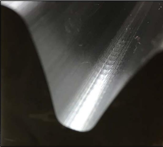
Figure 6 Chatter on gear tooth.
