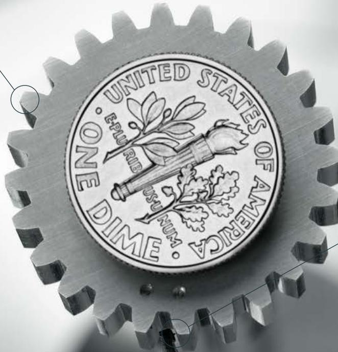
Klingelberg stylus for measuring roughness on small gears (Pat. pending)
