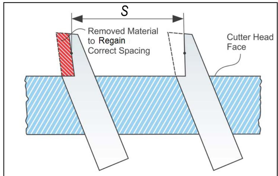
Figure 15 Regaining of correct blade spacing.
