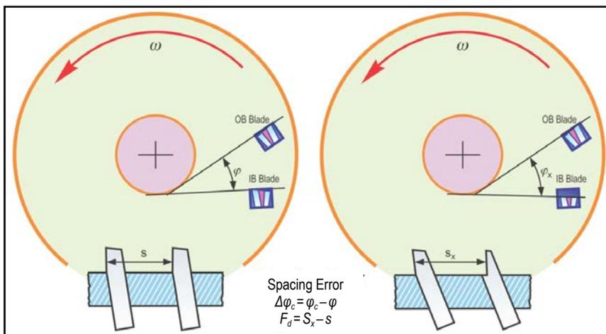
Figure 13 Cutting edge spacing  $\varphi$ .
