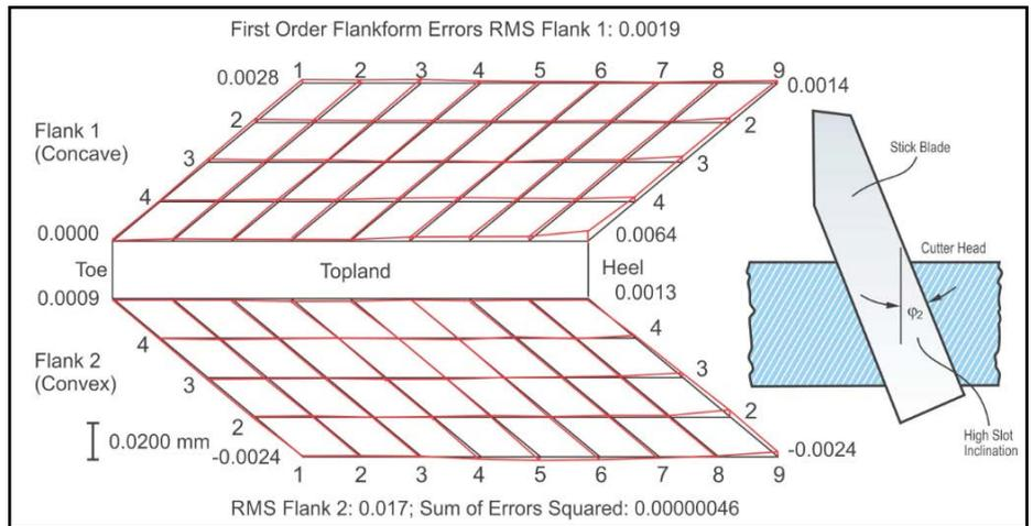
**Figure 21** Standard *CAGE* download file, part cut with  $12^\circ$  cutter slot inclination and 3-face blade with bade calculation after software revision.
