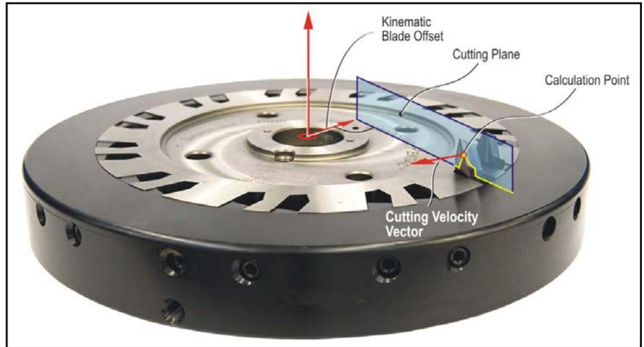
Figure 3 Cutting plane and kinematic velocity vector.
