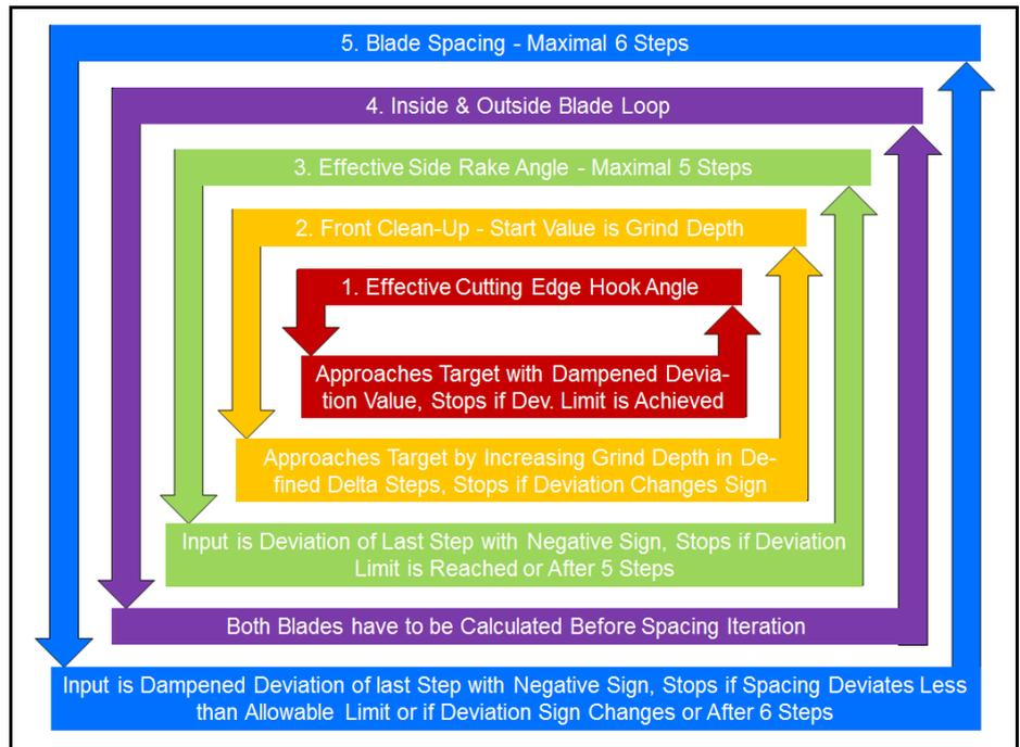
Figure 14 Five imbedded loops for 3-face blade calculation.
