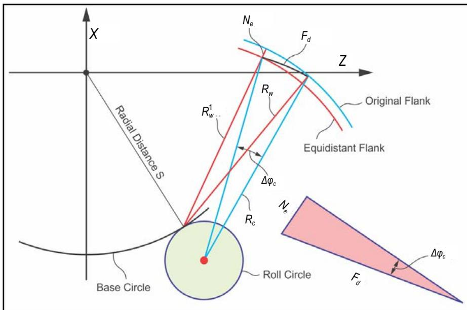
Figure 10 Radial compensation of spacing discrepancy  $F_d$ .
