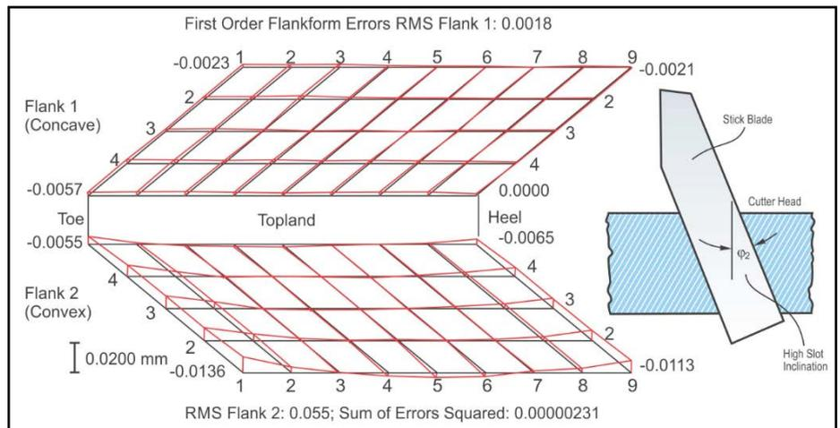
**Figure 19** Standard *CAGE* download file, part cut with 12° cutter slot inclination and 3-face blade with blade calculation before software revision.
