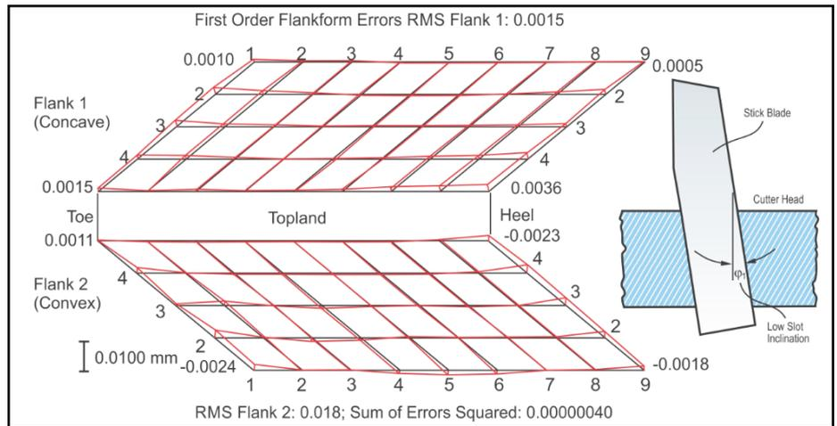
**Figure 18** Standard *CAGE* download file, part cut with 4.42° cutter slot inclination and 2-face blade.
