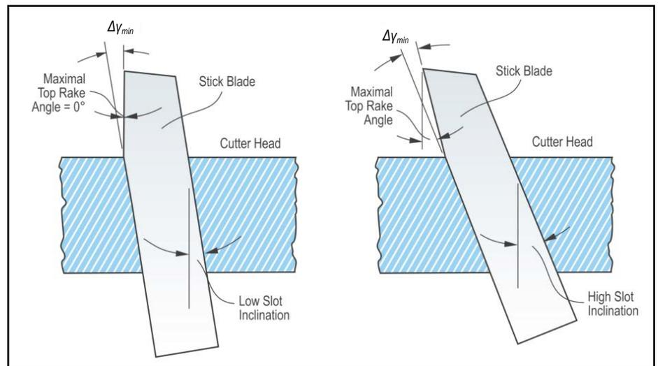
Figure 1 Top rake angle as function of slot inclination (slot tilt angle).
