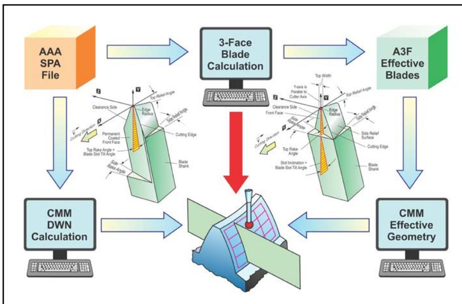
Figure 17 Two-face vs. three-face nominal CMM data file.
