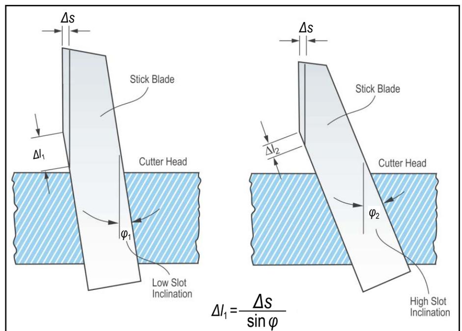
Figure 2 Relationship between top down amount and blade hook angle.
