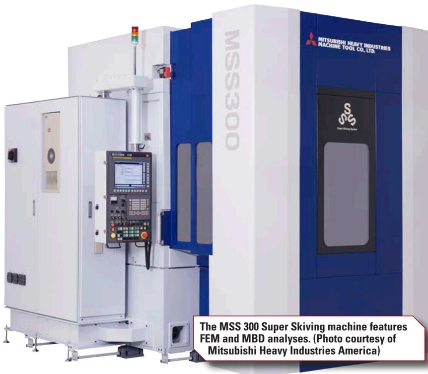
The MSS 300 Super Skiving machine features FEM and MBD analyses. (Photo courtesy of Mitsubishi Heavy Industries America)
