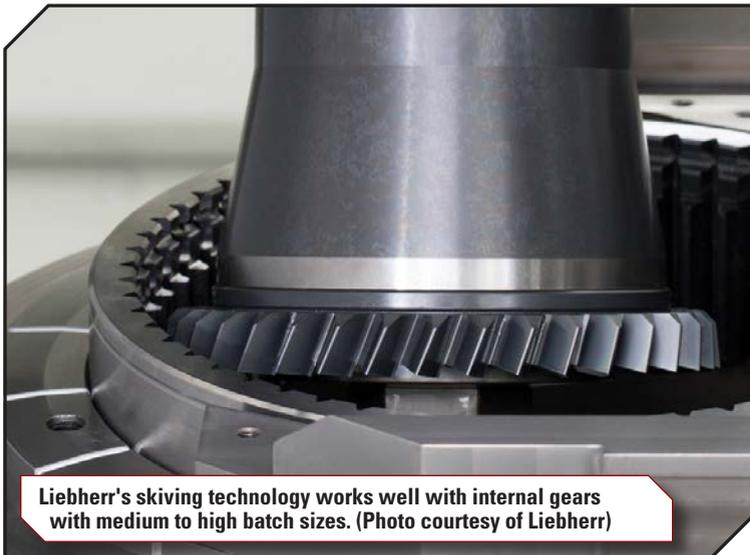
**Liebherr's skiving technology works well with internal gears with medium to high batch sizes. (Photo courtesy of Liebherr)**
