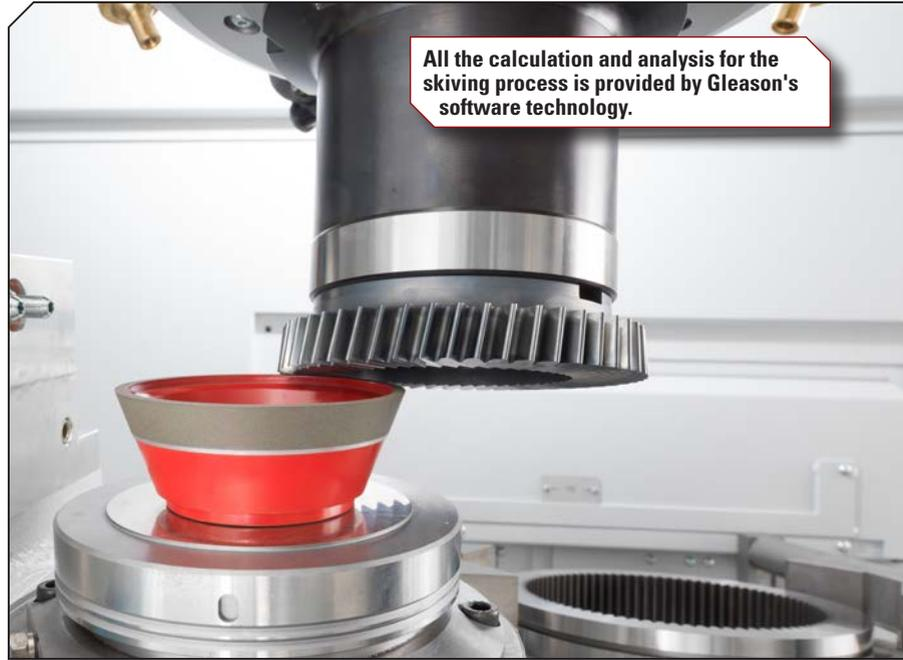
Frequent cutter changes are no longer required, a single cutter can stay on the machine for several days or weeks before it is fully used up. The time that has been used in the past by the operator for a cutter change is now being used for three to four automatic cutter grinding cycles with a reduced stock removal per grinding cycle to keep the cutter constantly sharp for a high and constant gear quality, he added.
