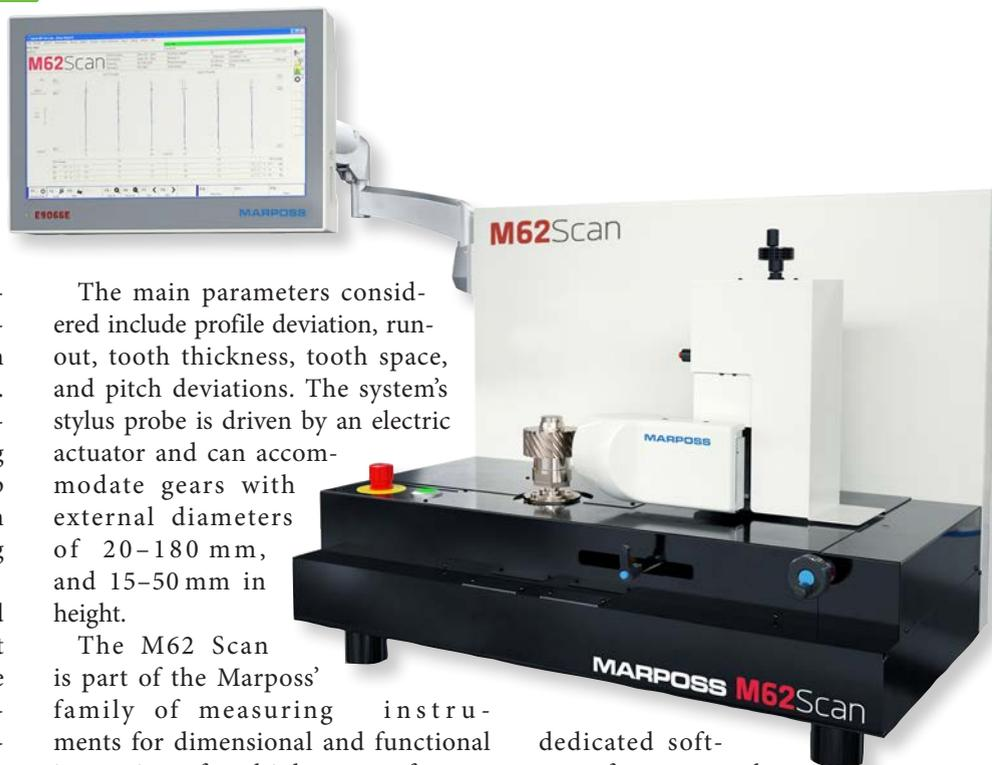
The main parameters considered include profile deviation, run-out, tooth thickness, tooth space, and pitch deviations. The system's stylus probe is driven by an electric actuator and can accommodate gears with external diameters of 20–180 mm, and 15–50 mm in height.
