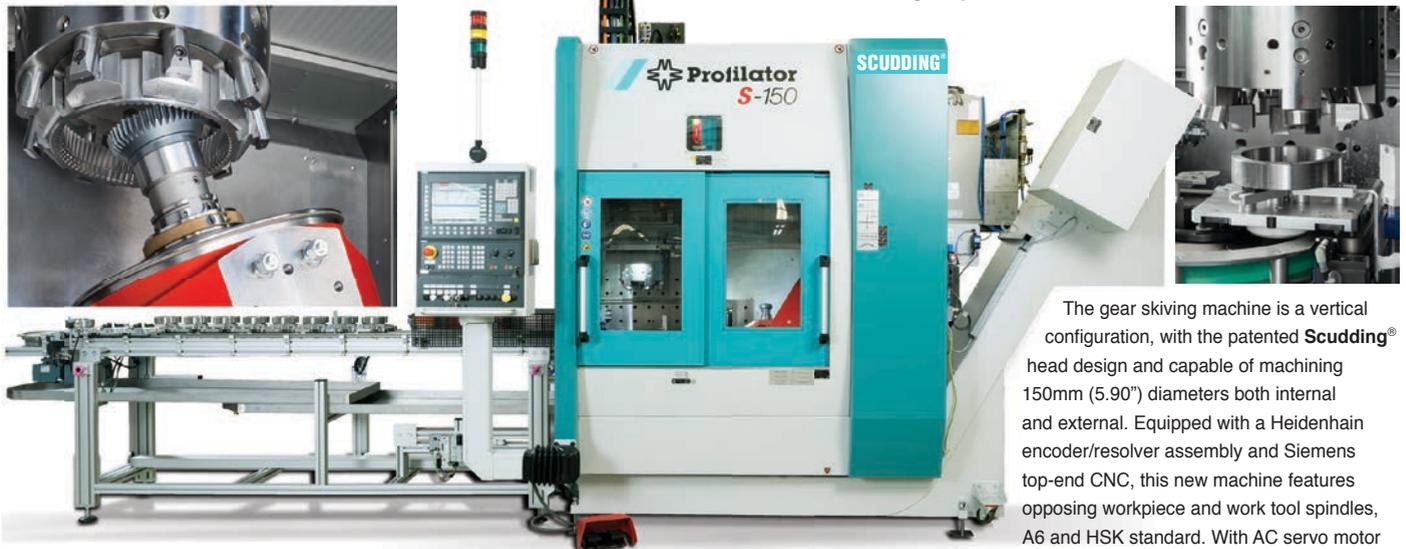
The gear skiving machine is a vertical configuration, with the patented Scudding® head design and capable of machining 150mm (5.90”) diameters both internal and external. Equipped with a Heidenhain encoder/resolver assembly and Siemens top-end CNC, this new machine features opposing workpiece and work tool spindles, A6 and HSK standard. With AC servo motor
