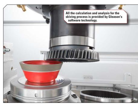
Frequent cutter changes are no longer required, a single cutter can stay on the machine for several days or weeks before it is fully used up. The time that has been used in the past by the operator for a cutter change is now being used for three to four automatic cutter grinding cycles with a reduced stock removal per grinding cycle to keep the cutter constantly sharp for a high and constant gear quality, he added.
