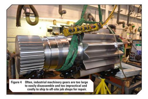
"In this application the SIFCO Process has extended the working life of the gear and improved the failure rate due to the nature of the nickel coating on the journal. The cost of manufacturing and material to replace the gear would have been exorbitant in comparison — as well as causing weeks of downtime."
