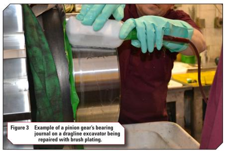
popular, while certain alloys like nickel tungsten alloys or nickel cobalt alloys can provide their own unique properties. With proper selection of deposition parameters, the grain structure of the nickel can be influenced to yield the desired properties such as hardness and corrosion resistance—thus enabling it to withstand the day-to-day operation that gears are subjected to.
