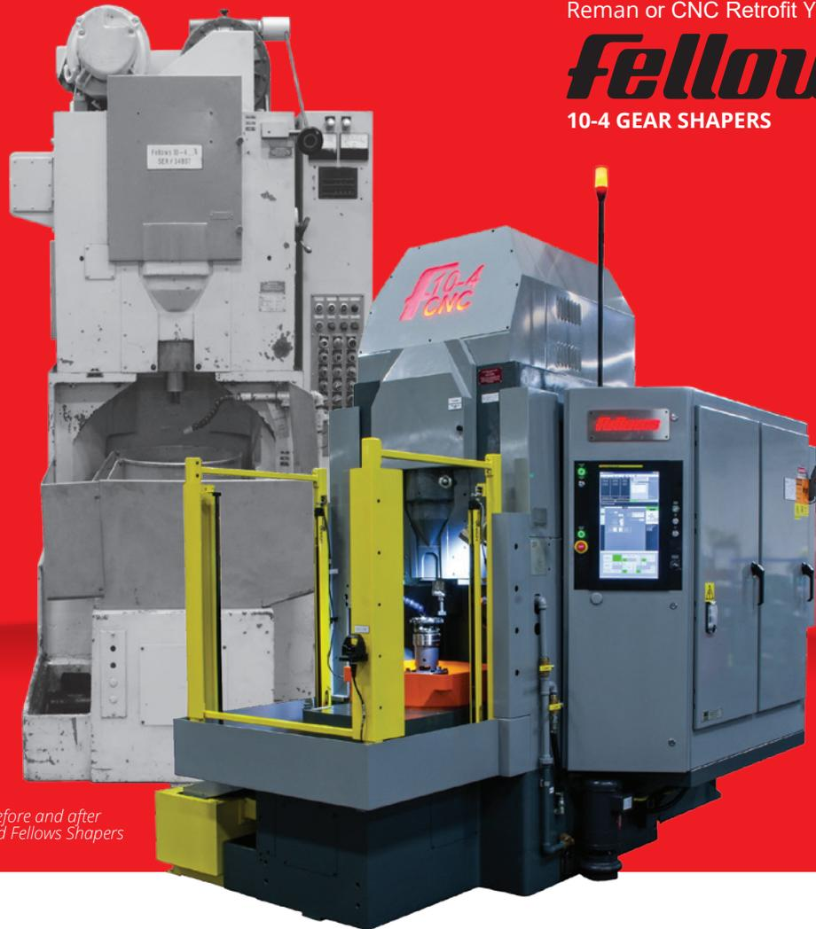
*Photos show before and after remanufactured Fellows Shapers*
