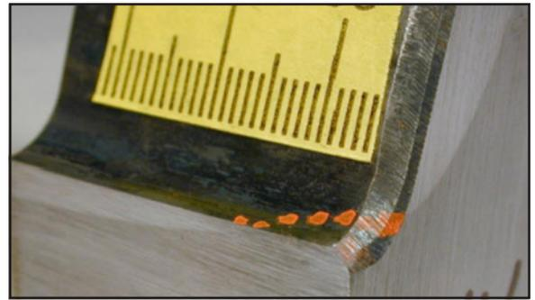
Figure 5 Unhardened area at end of tooth.
