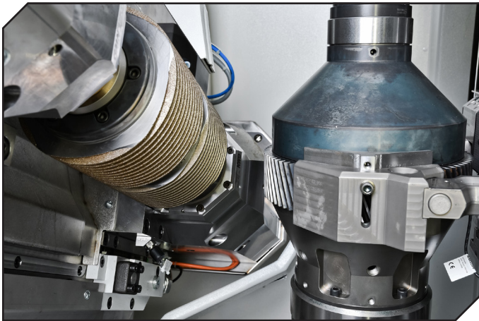
Generating grinding example of a drive gear for an e-drive with dressing-free CBN.
