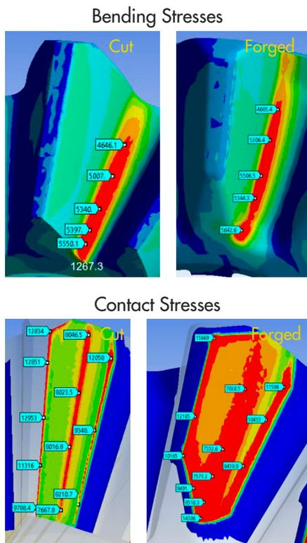
Torque on one side gear = 5,000 Nm
