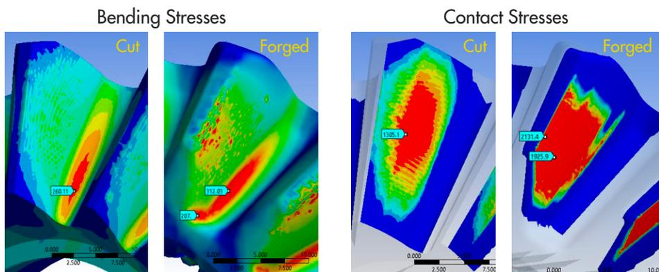
Torque on one side gear = 200 Nm
