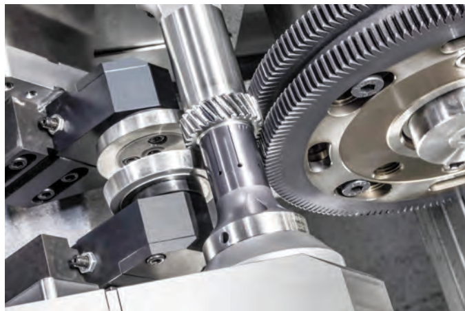
Chamfer rolling with secondary deburring discs. A very fast process that can, however, form a secondary burr that must be removed downstream.
