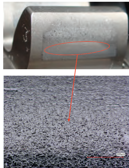
Figure 14—Appearance of micropitting on test gears after 67,500 cycles.
