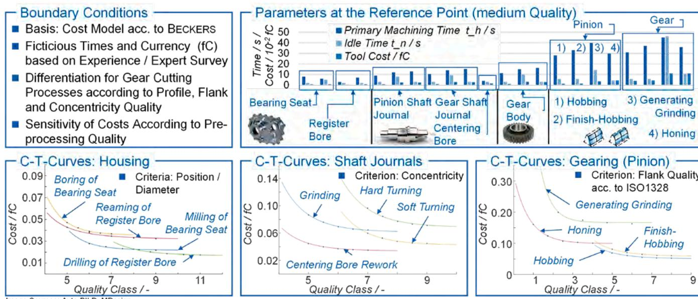
Figure 5—Process parameters in the reference point for calibrating the C-T curves.
