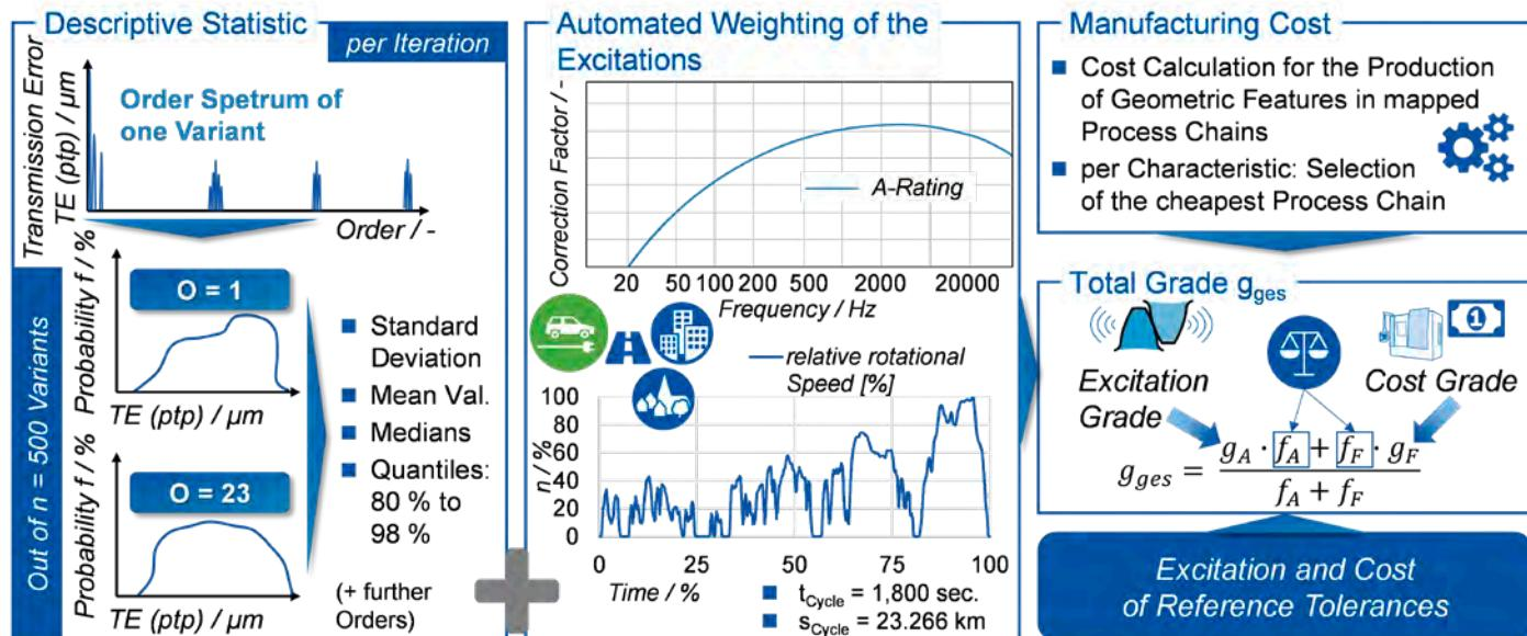
Figure 6—Determination of the overall grade on the basis of statistical transmission error parameters, a speed profile, the acoustic evaluation curve and the manufacturing costs.
