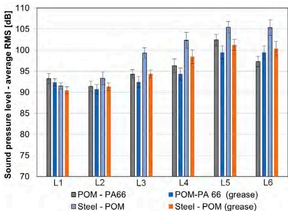
Figure 13—Comparison between measured sound pressure level for dry-run and grease-lubricated tests.
