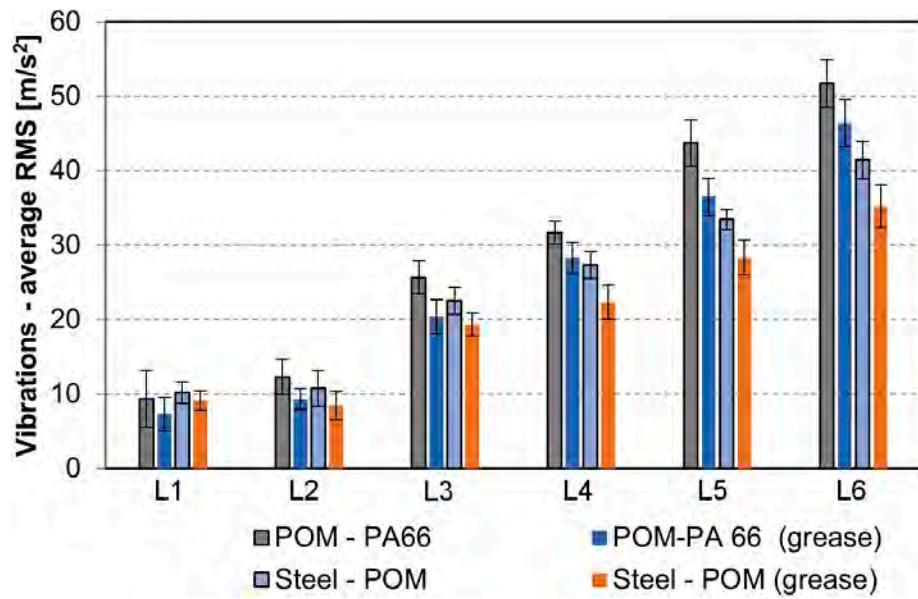
Figure 14—Comparison between measured vibrations for dry-run and grease-lubricated tests.
