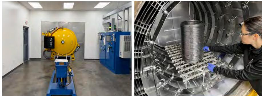
create an ultra-clean processing environment that meets the stringent demands of the aerospace and medical industries. Capable of achieving vacuum levels below  $5 \times 10^{-6}$  Torr, the system ensures bright, contamination-free results.
