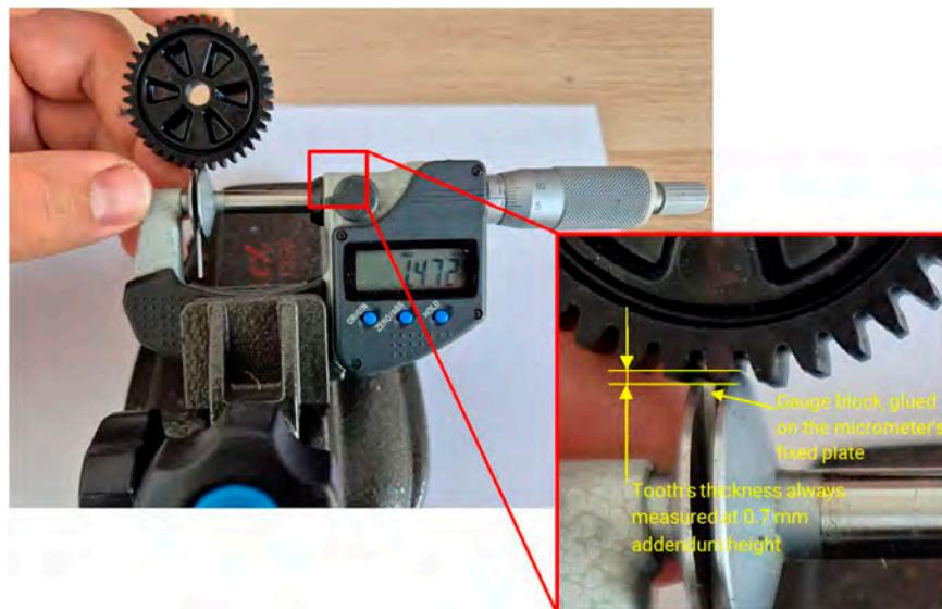
Figure 11—Wear measuring method—measured is the reduction in tooth thickness at the selected addendum height.
