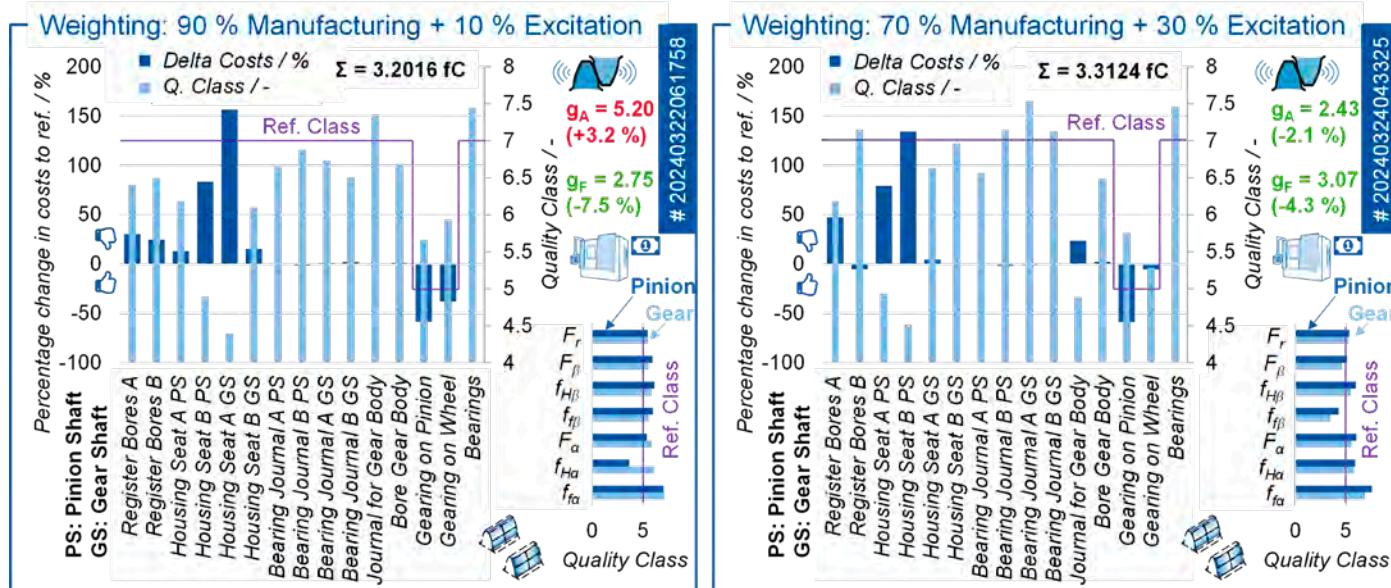
Figure 12—Quality and cost characteristics of two differently weighted tolerance designs.
