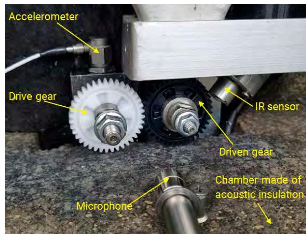
Figure 6—NVH testing set-up.
