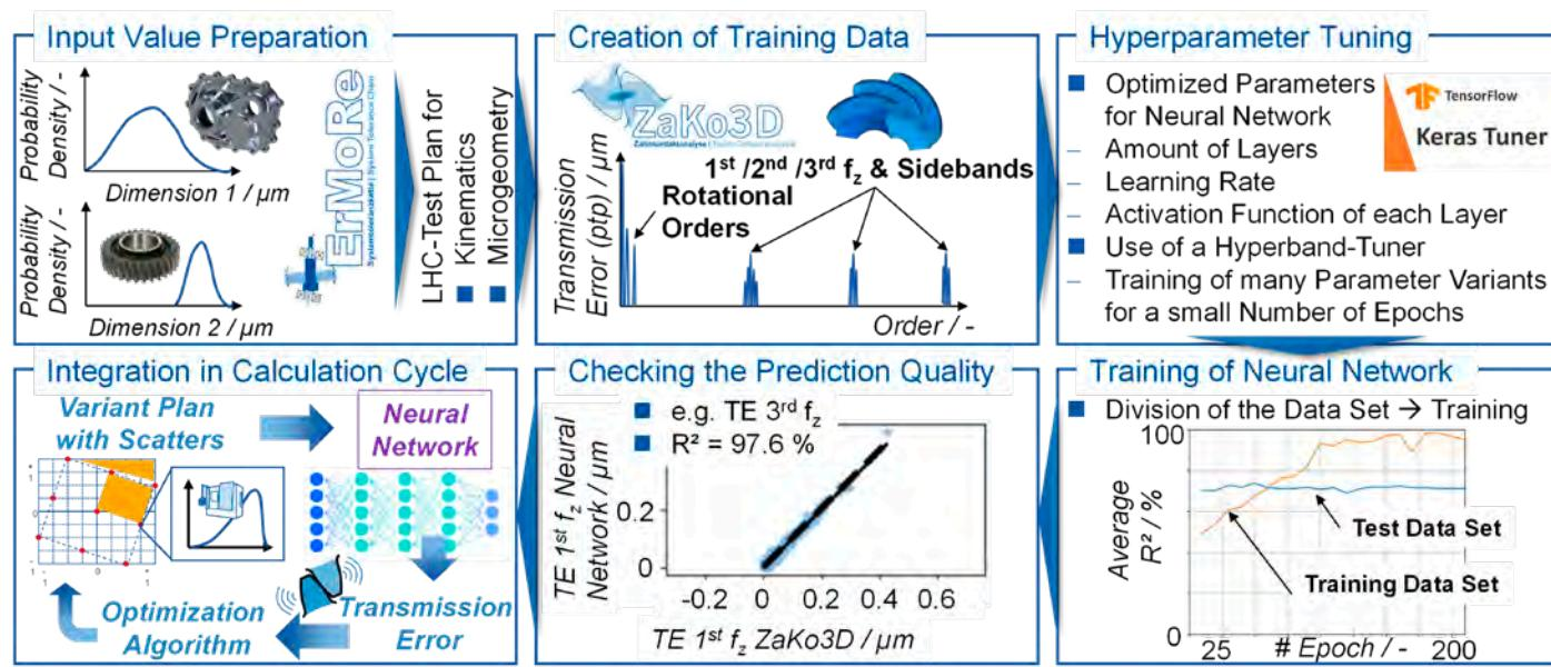
Figure 7—Procedure for increasing the performance of the calculation system with a meta model.
