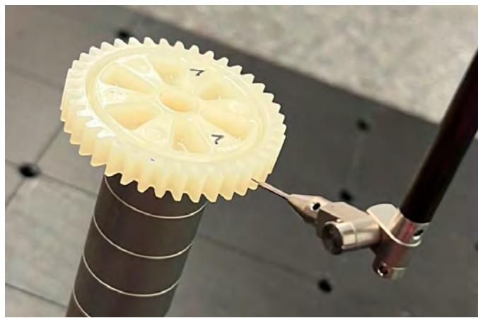
Figure 3—Geometric quality inspection on the plastic gear sample.
