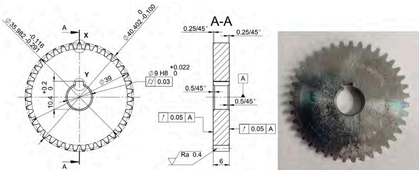
Figure 2—Steel gear samples employed for testing.
