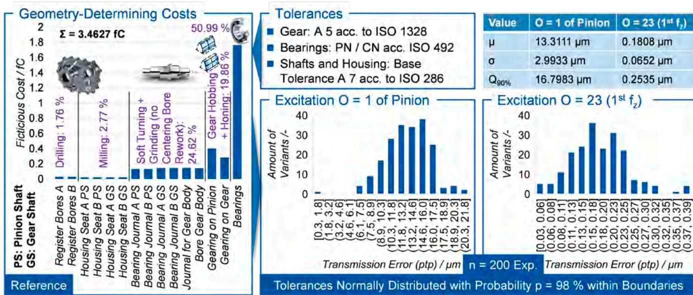
Figure 10—Geometry-determining costs and excitation distributions of the reference design.
