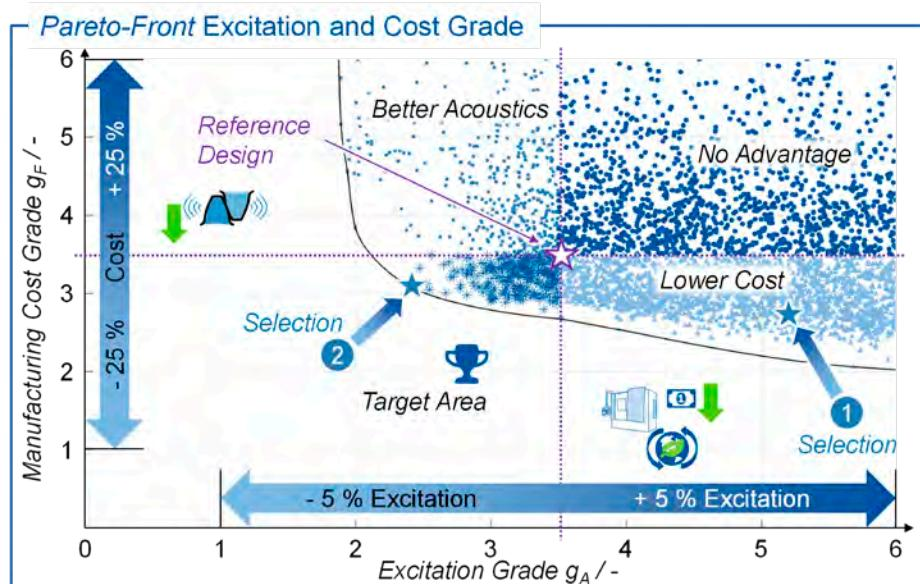
Figure 11—Pareto-Front generated with MOPSO and variant position of the target layouts.
