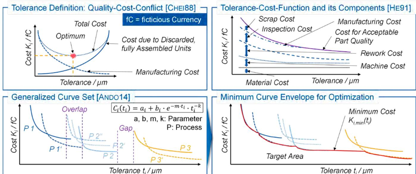
Figure 1—Quality-cost conflict, tolerance-cost function with its components and derivation of minimum costs according to Refs. 8–10.
