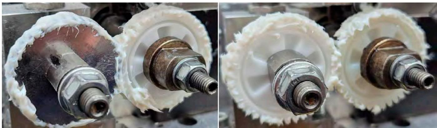
Figure 5—Grease applied on the gear pair before the tests in grease-lubricated conditions. (Left: Steel—POM gear pair; Right: POM—PA66 gear pair.)
