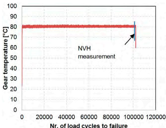
Figure 4—The gear's temperature and the transmitted torque were precisely controlled during each test. NVH measurements were done when 105 load cycles were reached.
