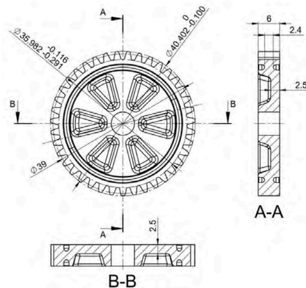
Figure 1—Plastic gear samples employed for the testing procedures.
