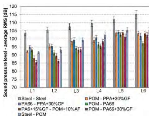
Figure 8—Sound pressure level, measured for the tested gear pairs. The temperature of plastic gears was controlled at 80°C in all tests (temperature measured on the teeth).
