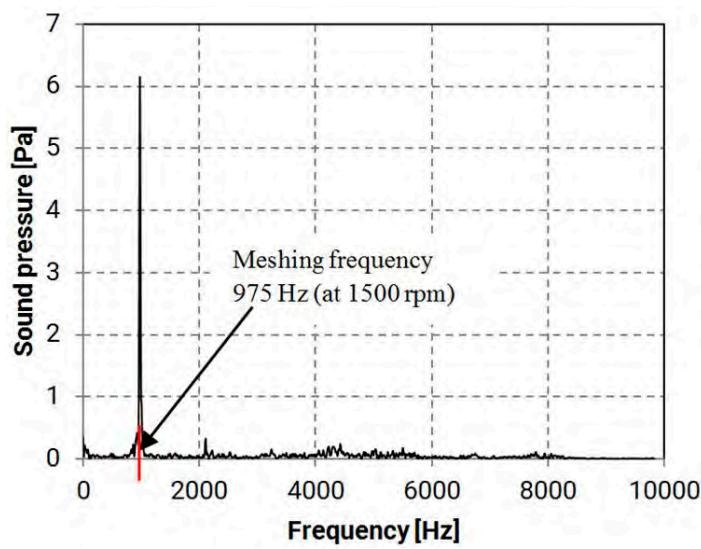
Figure 10—FFT of the measured vibrations and sound pressure signal. The rotational speed of the test was 1,500 rpm.
