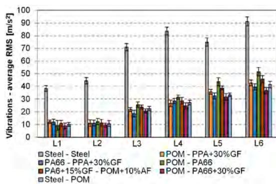
Figure 9—Vibrations, measured for the tested gear pairs. The temperature of plastic gears was controlled at 80°C in all tests (temperature measured on the teeth).
