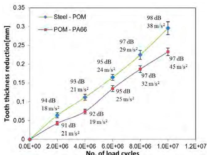
Figure 12—Average measured NVH in respect to the average wear measured for the tested gear pairs. Test conditions: 1,400 rpm, 2.0 Nm, 80°C.
