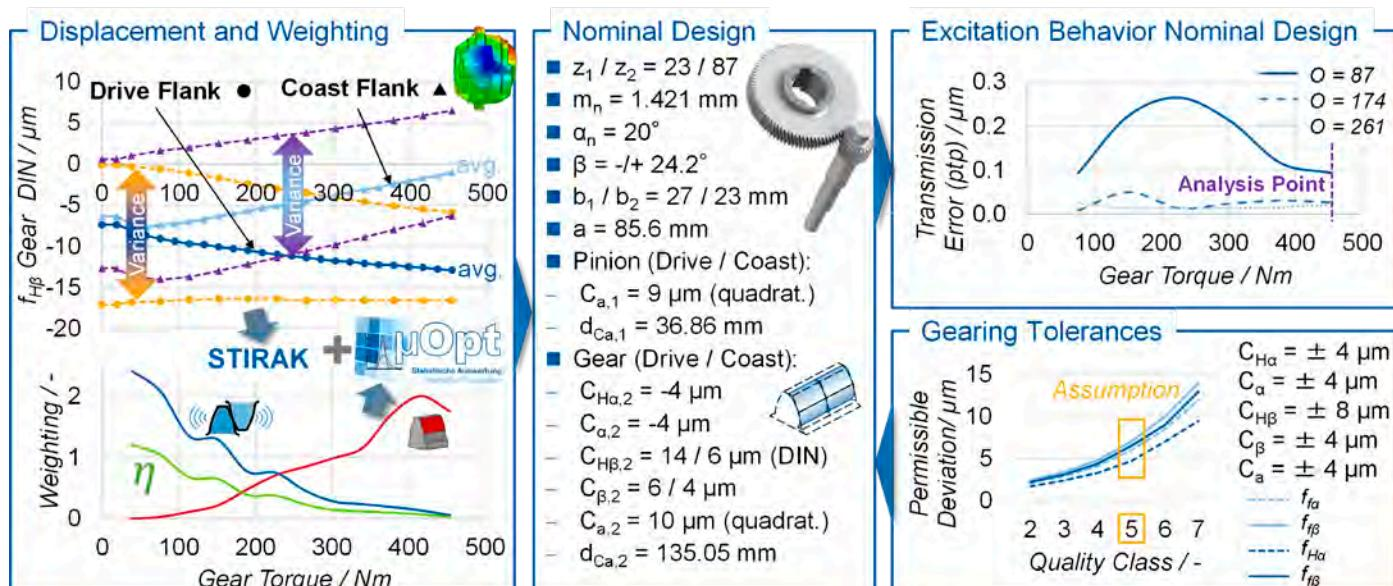
Figure 9—Consideration of misalignment behavior, weighting and gearing tolerances to identify the nominal microgeometry.
