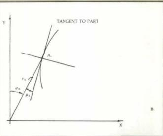
$$x_{c} = -\frac{r_{w}}{i} \times \sin(\psi_{P} \times i) + \frac{r_{A} \times \sin \sigma_{P}}{\cos \alpha} \times \cos(\alpha + \psi_{P} \times i)$$
