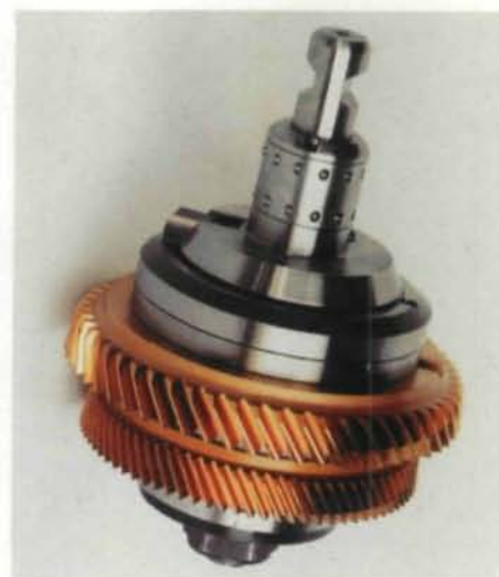
Fig. 12B—Cutter adapter with ball cage for concentric location of cutter to cutter spindle.
