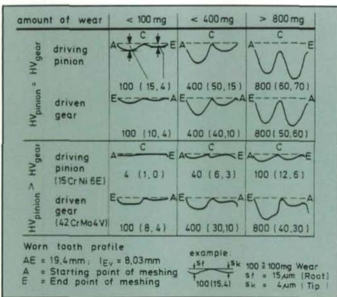
Fig. 5—Alteration of tooth profile along the path of contact for different amounts of wear and two material combinations (casehardened/casehardened and casehardened/through hardened gears).
