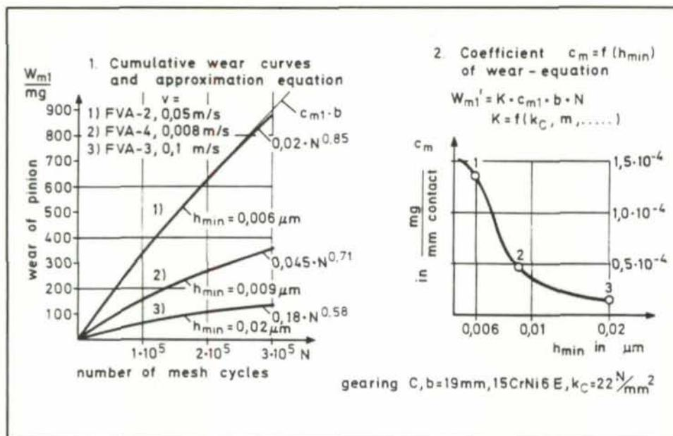
Fig. 7—Evaluation of wear coefficient  $c_m$  from wear curve. (Example for tooth form C according table 1).
