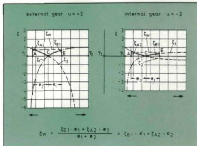
Fig. 10—Wear relevant specific sliding  $\zeta_W$ .
