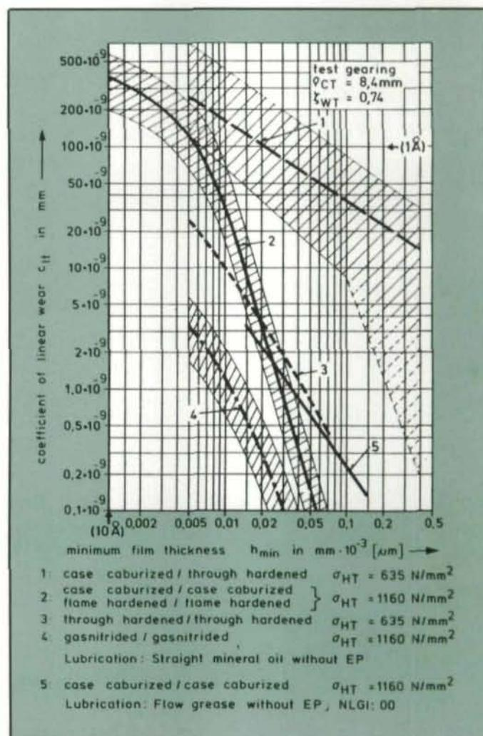
Fig. 8—Linear wear coefficient  $c_{lT}$  of the test gears depending on the EHL film thickness for different material combinations and lubrication conditions.
