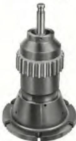
Drewco Hobbing Fixtures maintain the required close relationship between the locating surface and the face of the gear. The rugged precision construction maintains the close hold to face relationship whether locating on smooth diameters or spline teeth. The expanding arbor will effectively hold a gear blank for finish turning, gear cutting, gear finishing, and gear inspection operations.
