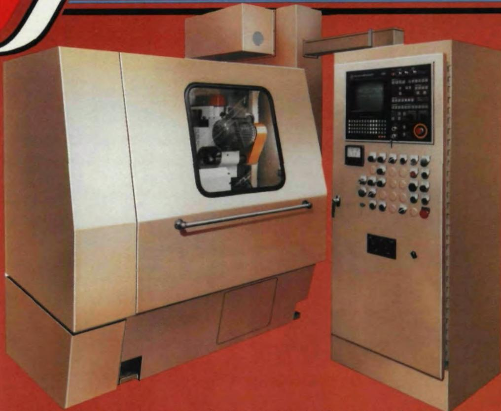
These domestically manufactured machines have fully programmable automatic grinding cycles and user needs are fully accommodated in their design. We provide on-site engineering service and training to our customers.
