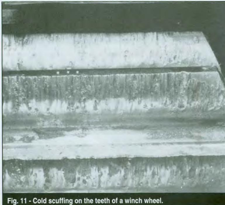
**Fig. 11 - Cold scuffing on the teeth of a winch wheel.**
