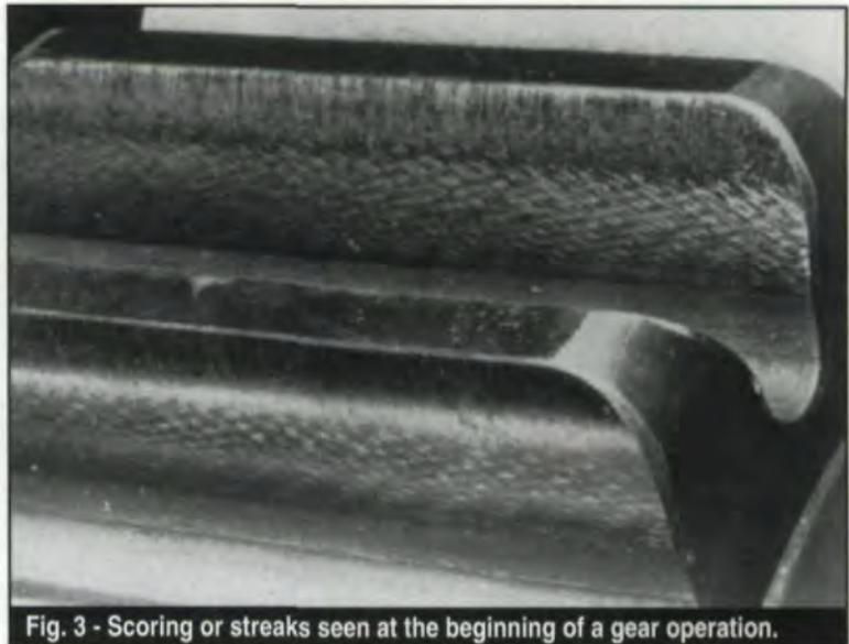
Fig. 3 - Scoring or streaks seen at the beginning of a gear operation.
