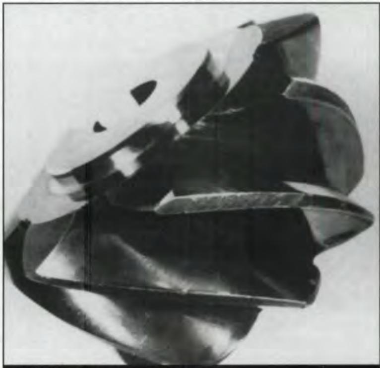
Fig. 6 - Polishing on a spiral bevel gear.
