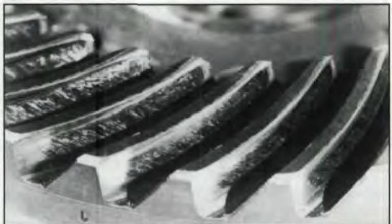
Fig. 9 - Destructive scuffing on the teeth of a spiral bevel wheel. Note the presence of deep streaks and important deformations of the profile in the contact zones. This gear wheel can be considered as destroyed.
