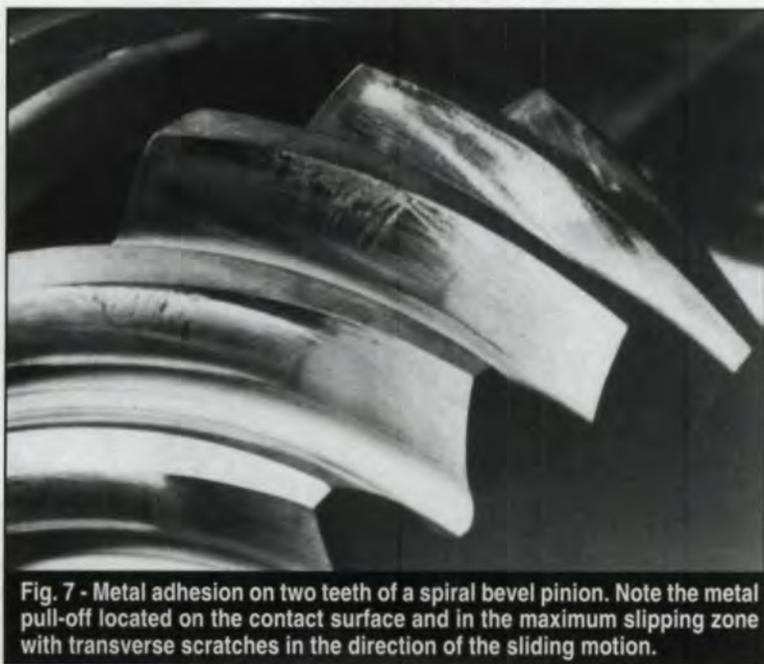
Fig. 7 - Metal adhesion on two teeth of a spiral bevel pinion. Note the metal pull-off located on the contact surface and in the maximum slipping zone with transverse scratches in the direction of the sliding motion.
