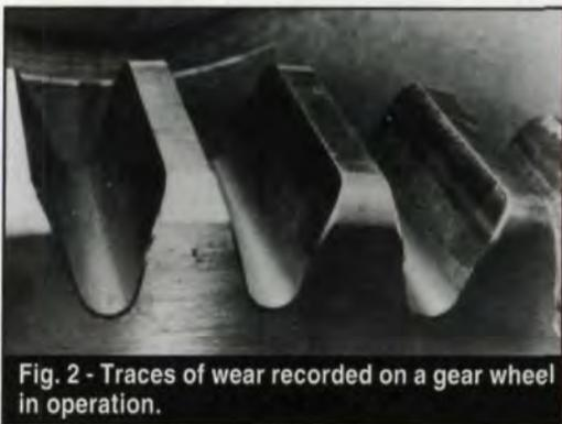
Fig. 2 - Traces of wear recorded on a gear wheel in operation.
