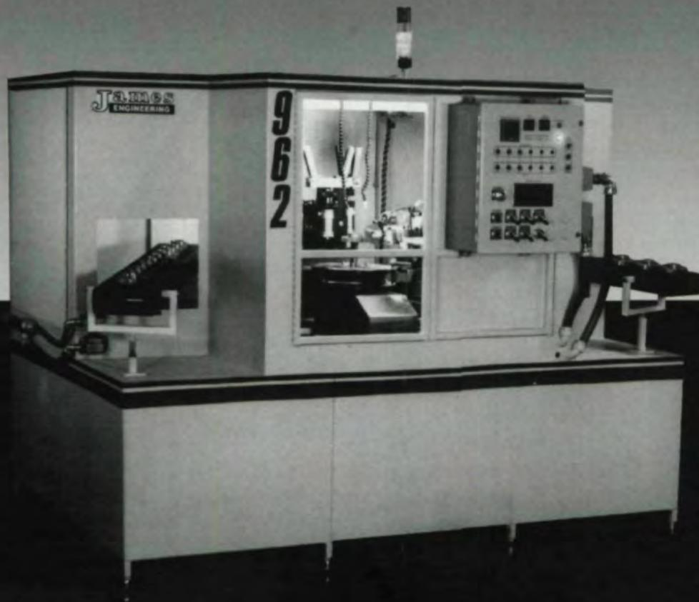
Over two years of intense development has been spent on the revolutionary **962 ADS System**. New Technology (Pat. Pend.) has been developed to allow precision high volume deburring automatically. No operator is needed except to replenish the tool reservoir after approximately 26,000 parts have been deburred. Reloading tool system takes only a few minutes. Computer controls feature a self diagnostic system, a part process monitoring and CIM communications.
