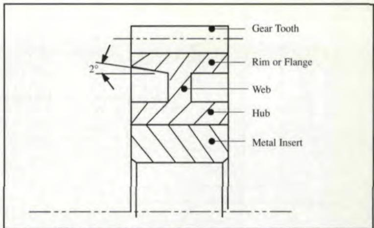
Fig. 2 — General features of nonmetallic gears.
