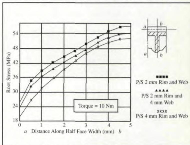
Fig. 9 — Effect of web thickness on bending stress.
