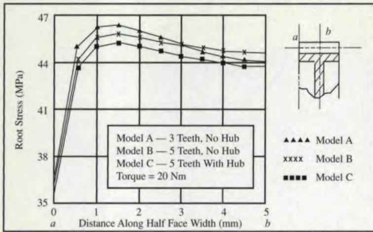
Fig. 5 — Variation of principal bending stress across the gear half face width for different finite element models.
