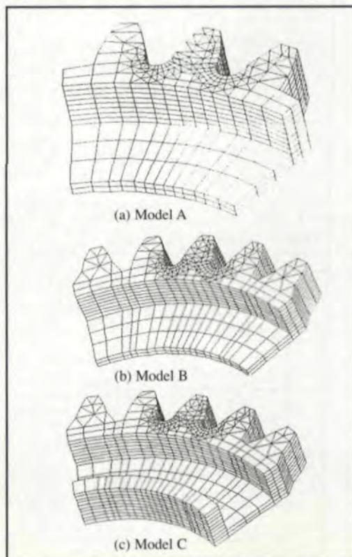
Fig. 4 — Various models of finite element mesh.
