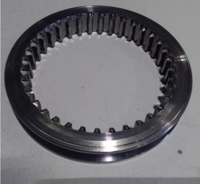
Steel: 20NiCrMo Diameter:150 mm
