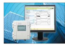
The HOBO U30/ETH remote monitoring system, from Onset Computer Corporation, is an industrial grade system that monitors energy and provides real-time, remote access to facility energy and environmental data over an Ethernet connection.
