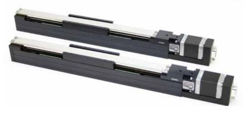
the assembly is a precision preloaded 8 mm diameter Steinmeyer ball screw, miniature size 9 linear guideway, noncontact limit switches and a choice of either stepper motor or DC servo motor with encoder. A separate motion controller is an available option.
