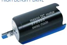
The RE 50 from Maxon motor features an ironless rotor, which results in detent-free running and minimized mass inertia. The drive combines a two-pole neodymium permanent magnet with Maxon's patented winding technology for high torque and acceleration.
