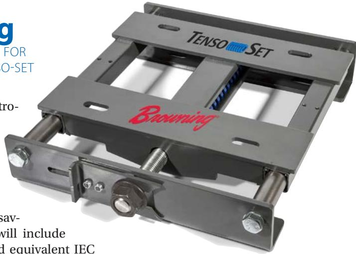
the belt. However, the Tenso-set base includes a coil spring inside the screw housing that pushes against the carriage to maintain tension as the belt naturally breaks-in and seats itself further into the sheave groove due to loss of mass.
