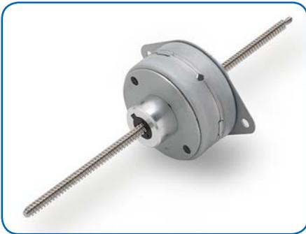
With a holding force of 112N, the 35DBM stepper linear actuator is suited for use in applications such as auto injectors, laboratory automation, medical pipettes and valve actuation. Portescap's 35DBM high-force actuators are fully customizable for adaptor tips, stroke lengths, windings, flanges and end of motion detection sensors.
