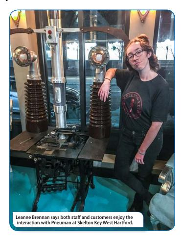
and receiving stations. An air compressor/motor pump is installed at the receiving station which can suck (like a vacuum cleaner) or blow air. When it sucks air, it pulls loaded canisters along the tube toward it. When it blows air, it *pushes* the canisters in the opposite direction. The tubes can go along straightaways or easy curves to cover the areas of necessary travel.
