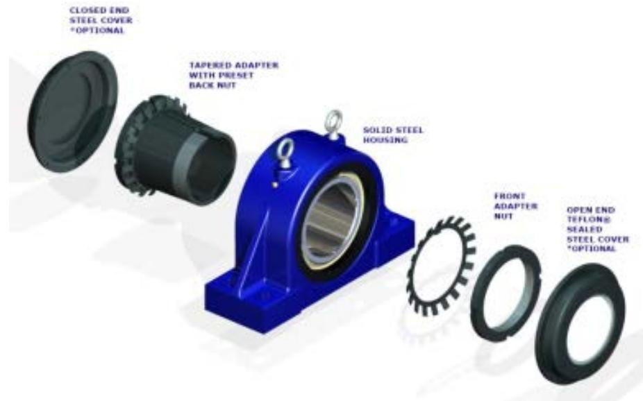
adapter sleeve (with front lock nut) to include a mechanical withdrawal nut on the back end that is factory set for nominal shaft sizes and, if necessary, can be easily adjusted in the field to accommodate actual (under/over) shaft size.
