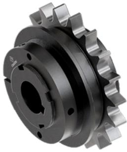
*The EDF/F series is a ball torque limiter, which consists of two halves: a driving member and a driven member that are separated by a set of steel balls housed in grooves on both members.*
