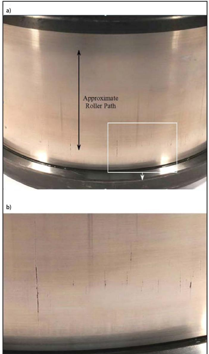
Figure 2 (a) Axial cracks on intermediate bearing INT-B IR; (b) axial cracks on intermediate bearing INT-B IR.
