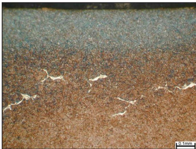
Figure 11 irWEAs on rotor bearing ROT-D IR.
