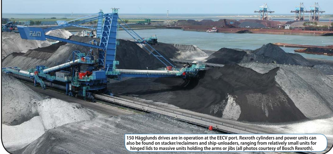
150 Hägglunds drives are in operation at the EECV port. Rexroth cylinders and power units can also be found on stacker/reclaimers and ship-unloaders, ranging from relatively small units for hinged lids to massive units holding the arms or jibs (all photos courtesy of Bosch Rexroth).
