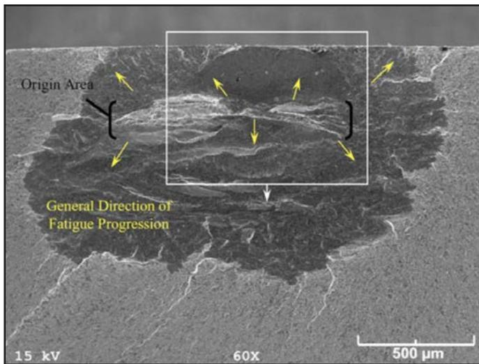
Figure 4 Opened axial crack on intermediate bearing INT-B IR.
