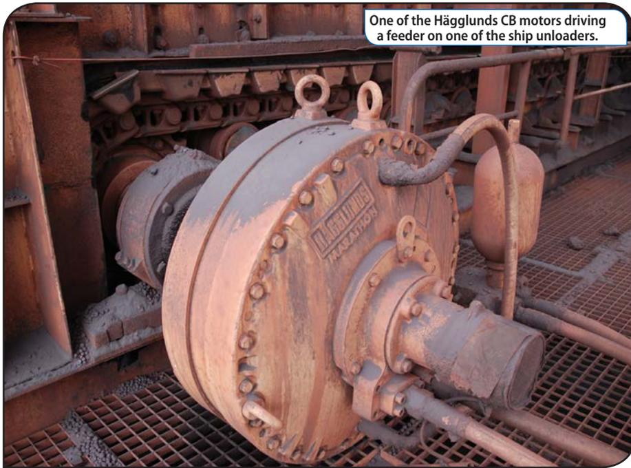
One of the Hägglunds CB motors driving a feeder on one of the ship unloaders.
