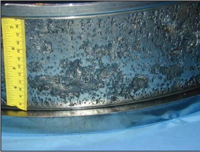
Figure 7 Macropitting on rotor bearing ROT-D IR.
