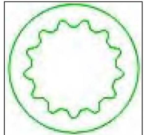
Figure 3 Splined bore.
