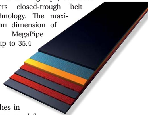
inches in diameter, while standard brands do not exceed an external diameter of 27.6 inches. Thus, the capacity of the conveyor system is increased by more than 100 percent compared to conventional closed-trough belts. With this new development, the ContiTech Conveyor Belt Group now provides an enclosed conveyor belt solution which can transport large lump sizes. MegaPipe can be utilized immediately after a primary crusher application.
