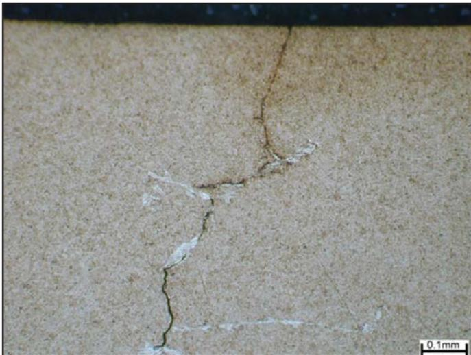
Figure 3 Irregular white etching areas on axial crack.
