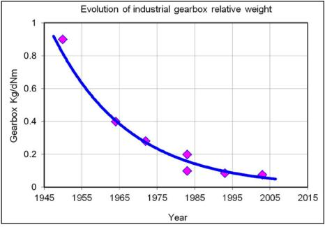
Figure 1 Typical relative weight evolution in industrial gearboxes during the last 50 years (Ref. 6).
