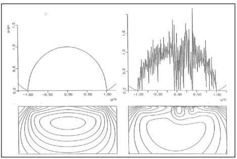
Figure 8 Example of stress field a) nominal smooth contact geometry, b) actual rough geometry (Ref. 27).
