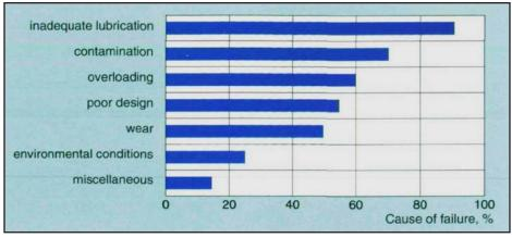
Figure 9 Causes of rolling bearing failure as percentage of responses from an enquiry among the companies of the FVA associations (Ref. 34).
