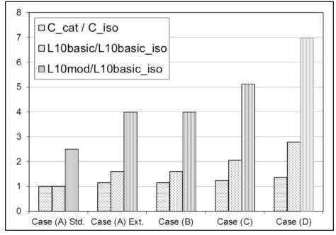
Figure 4 Overview of different dynamic rating rules found in the market place; to simplify the discussion, the life modification factor  $-a_{150}$  - is taken for all cases equal to 2.5.
