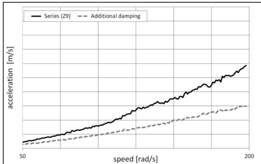
Figure 11 Additional damping | influence on vibration.
