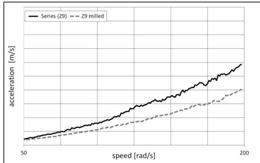
Figure 9 Manufacturing process | influence on vibration.
