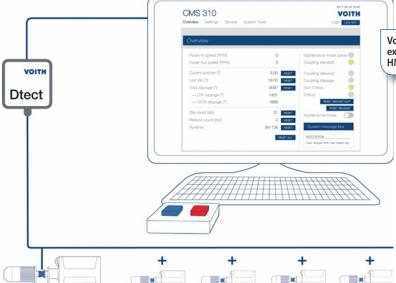
that it is performing. The accuracy and timeliness of the measurement will provide the operator the ability to maximize machine productivity without exceeding individual drive chain component capacities. In addition, equipment monitoring can provide the ability to produce trend data for each monitored component of the drive chain. This can help operators make decisions about the health of each drive component allowing them to order spare parts in preparation for repair.
