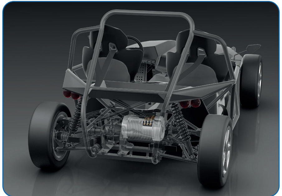
The optimized cooling is further supported by installing the drive transversally to the driving direction (courtesy of ABM).
