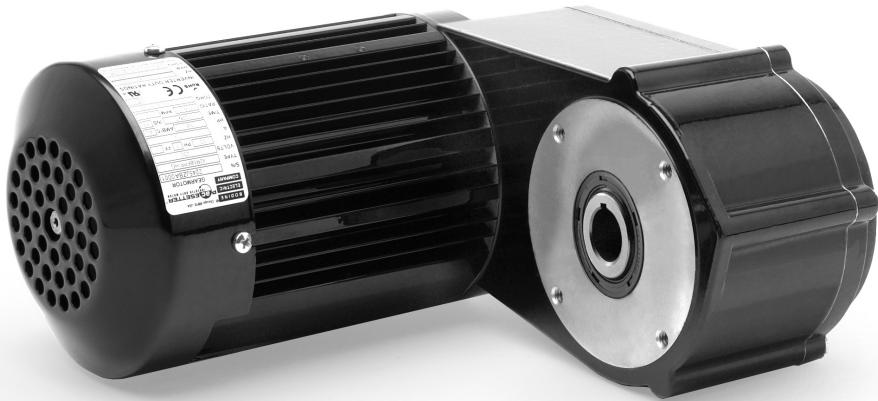
gearheads. The offset design allows the gearmotors to deliver high torque for their size through a range of gear ratios. The large center distance between the gearbox and the motor enables these units to be fitted with dual drive shafts. The HG/H gearbox also features large hardened helical and spur gears and needle bearings to ensure quiet, long-lasting operation.
