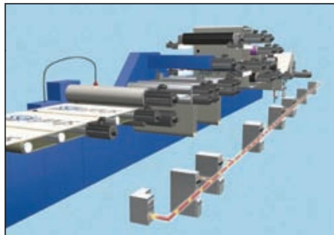
employ a high-speed AC servomotor, which moves each roller via a direct drive. Each servomotor provides precise control to within 0.0002", while moving at surface speeds of 1,560' per minute. Meanwhile, each servo drive can be networked together via fiber optic cabling, which enables tight synchronization between the drives.
