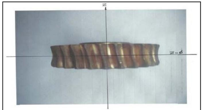
Figure 15 Single-enveloping worm gear.
