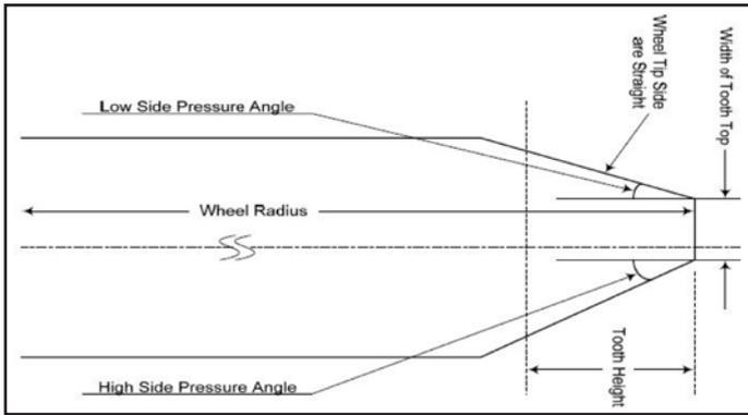
Figure 11 Grinding wheel geometry for Spiroid gear pinion.
