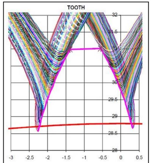
Figure 18 Axial cross-section of the gear tooth at *z*=3 mm.
