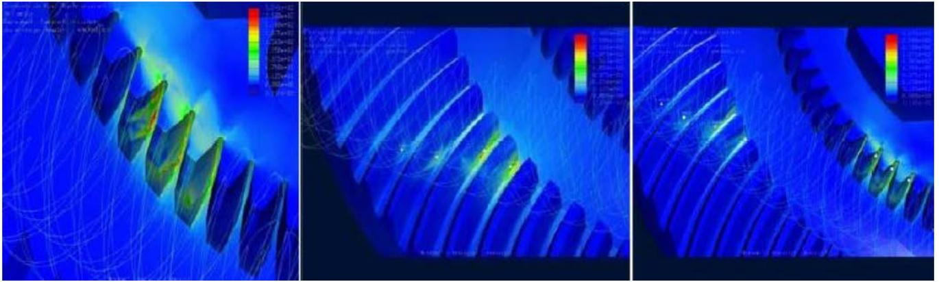
Figure 22 FEA outputs on the hybrid gear.
