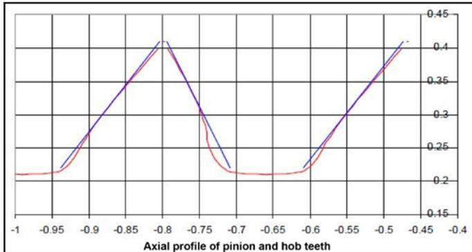
Figure 12 Pinion tooth (in red) inside the hob tooth (in blue).
