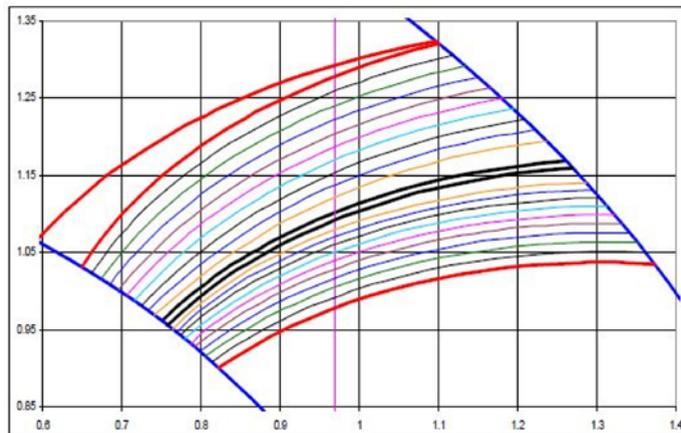
Figure 7 Gear groove profile with enhanced design using *Gearometry* software.
