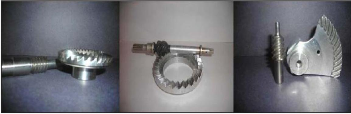
Figure 2 The three types of Spiroid gear.
