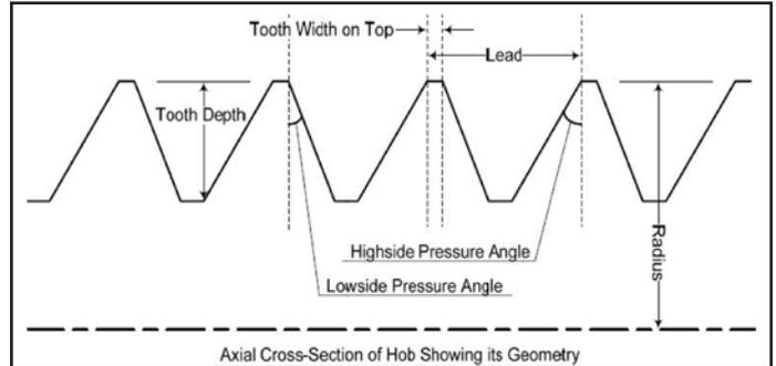
Figure 3 Axial cross-section of a cylindrical hob.
