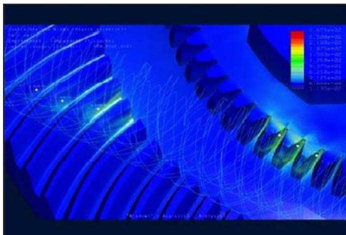
Figure 9 Example of FEA under load from *Gearometry* software data.
