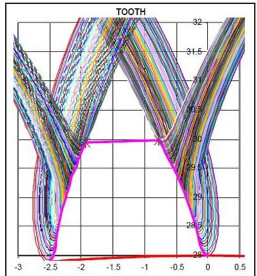
Figure 17 Axial cross-section of the gear tooth at *z*=0 mm.
