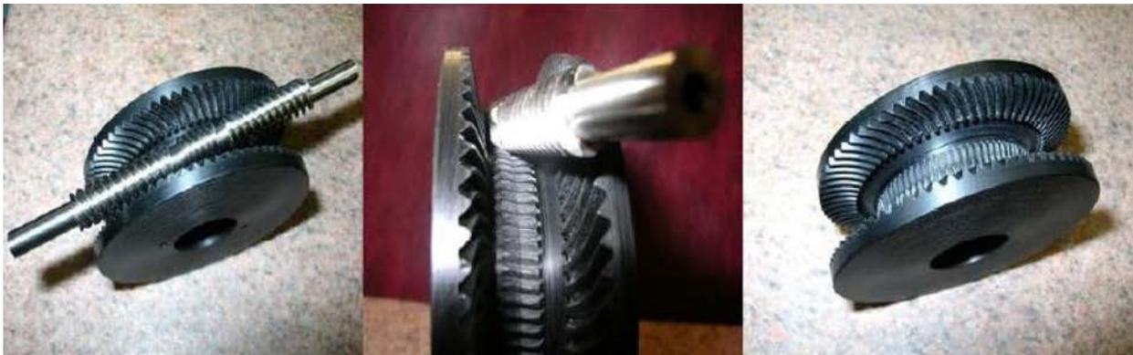
Figure 21 New “hybrid” gear made of a double-Spiroid gear, and worm gear driven by same pinion.
