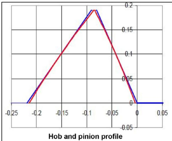
Figure 13 Pinion tooth (in red) with circular sides contained inside the hob tooth (in blue).
