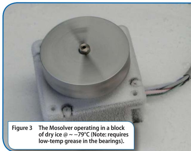
**Figure 3** The Mosolver operating in a block of dry ice @ ~ -79°C (Note: requires low-temp grease in the bearings).
