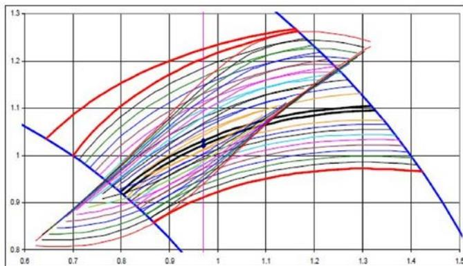
Figure 10 *Gearometry*-enhanced design gear groove with hob tooth superimposed.
