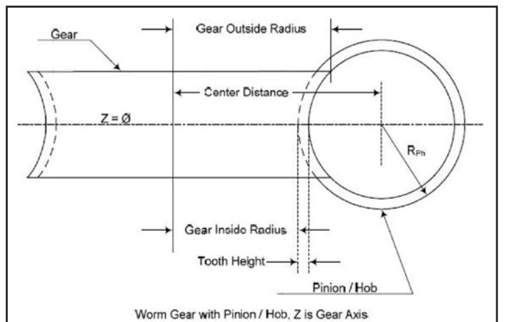
Figure 16 Worm gear/pinion assembly or gear/hob set-up.
