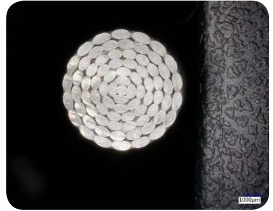
spray PTFE, ETFE, PU, PE, FEP with lubricity and bonding strength; centerless grind the distal end for multi-segmented flexibility; rotary swaging for torsional rigidity, and augering the drive cable with a stainless wire for additional cutting and aspirating capability.
