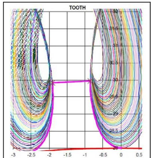
Figure 19 Axial cross-section of the gear tooth: at *z*=0 mm; lead=11 mm.
