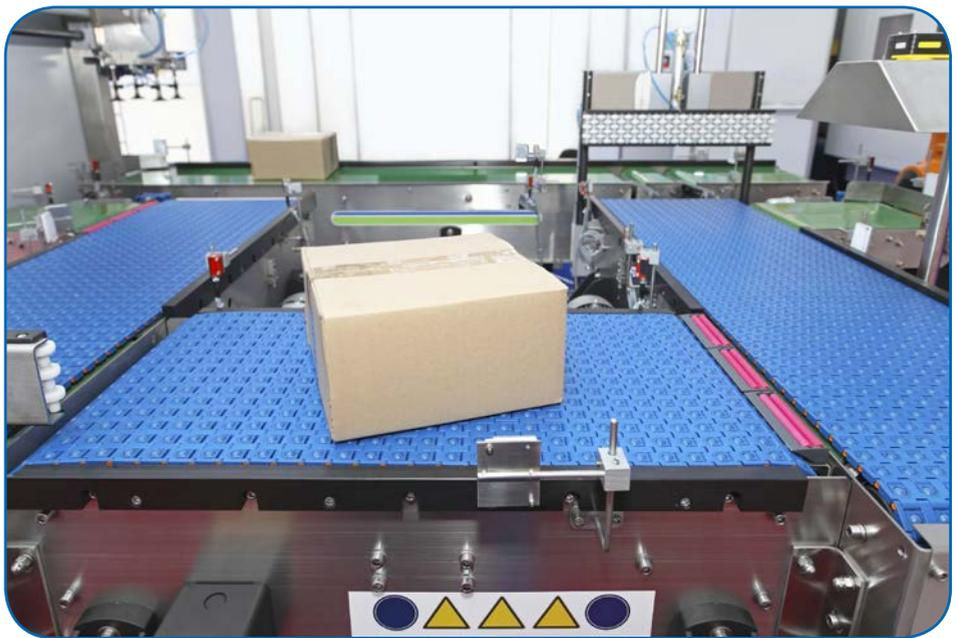
ft (9,000 Nm/m) or 1.1 lb/ball (0.5 kg/ball). The belt’s non-contact product manipulation eliminates impact and abrasion damage from pushers, as well as the need for mechanical adjustment or changeovers for conventional diverters or guides.
