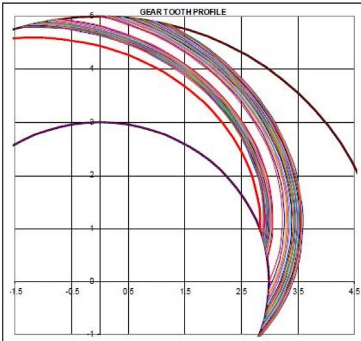
Figure 26 Spiral bevel gear groove with high-side and low-side profiles made of curves in conical surfaces parallel to root or top of the gear.
