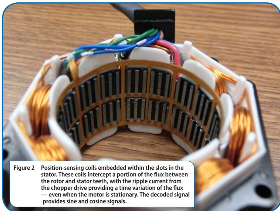
Figure 2 Position-sensing coils embedded within the slots in the stator. These coils intercept a portion of the flux between the rotor and stator teeth, with the ripple current from the chopper drive providing a time variation of the flux — even when the motor is stationary. The decoded signal provides sine and cosine signals.
