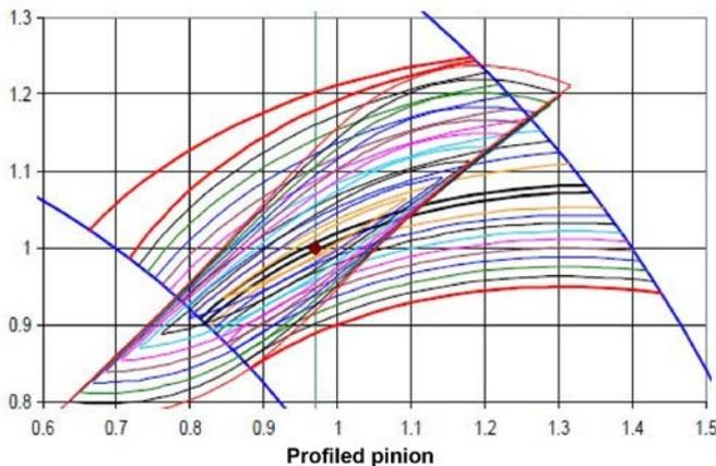
Figure 14 Circular sides pinion tooth superimposed inside the gear groove.
