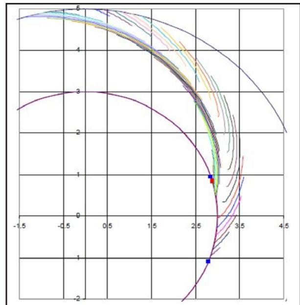
Figure 24 Axial cross-section of spiral bevel gear hob showing its geometry and parameters.
