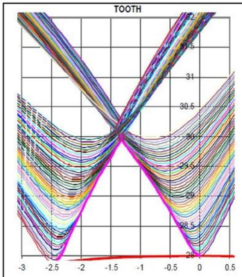
Figure 20 Axial cross-section of the gear tooth: at  $z=0\text{mm}$ ; lead=9mm.
