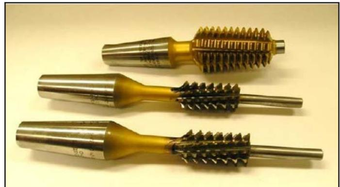
Figure 4 Cylindrical and tapered hobs.
