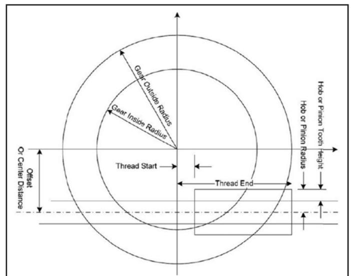
Figure 1 Spiroid gear/pinion assembly or gear/hob set-up.
