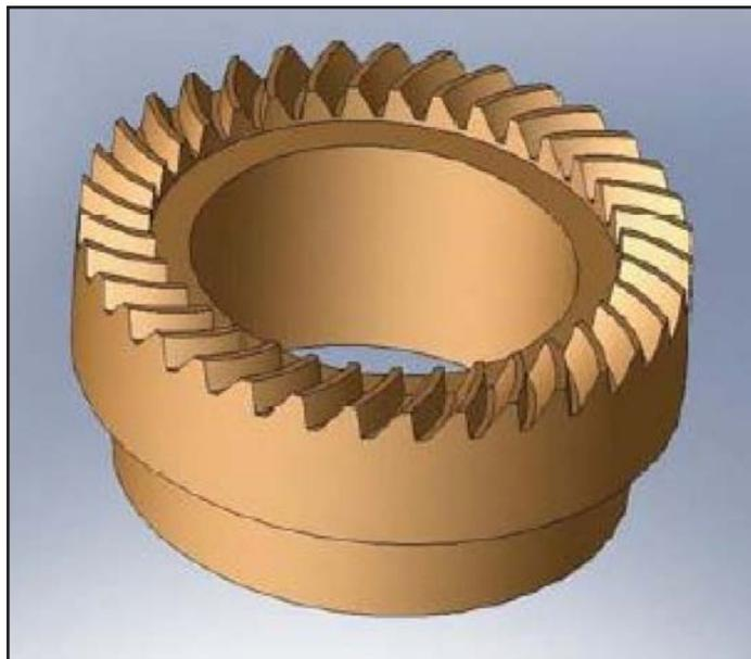
Figure 8 Example of true 3-D model of flat-face Spiroid gear from *Gearometry* software data.
