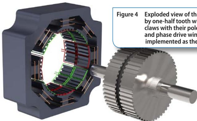
**Figure 4** Exploded view of the Mosolver. The rotor has two pole caps, with the north and south poles skewed by one-half tooth width; the magnet is between the pole caps and is axially magnetized. The stator claws with their pole teeth are also exposed, showing the location of both sensor windings (red, green) and phase drive windings (copper). The actual sensor windings have a multiple turns-per-coil, and are implemented as the flex circuit shown in Figure 2.
