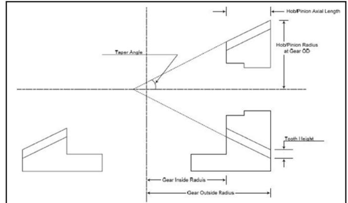
Figure 23 Spiral bevel gear set-up with hob or pinion.
