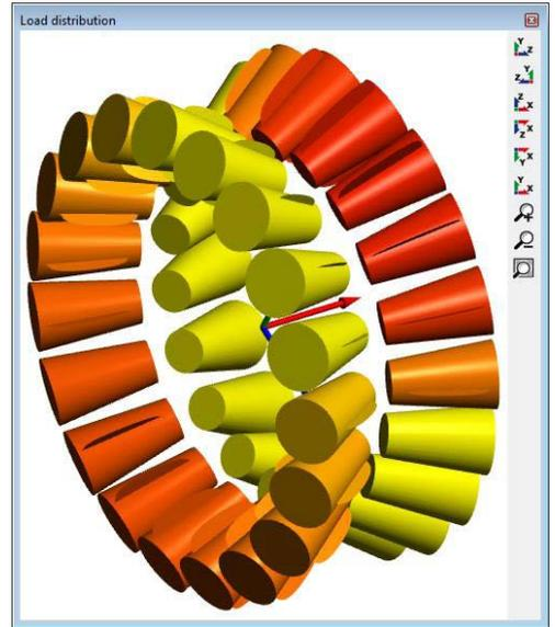
In addition to the shaft and rolling bearing calculation software a new calculation of load distribution for ball screws is available now. Life is calculated from load distribution analogously to ISO/TS 16281. This allows the consideration of radial and moment loads in addition to axial loads. As in the other programs, an automatic parameter variation is available as well.
