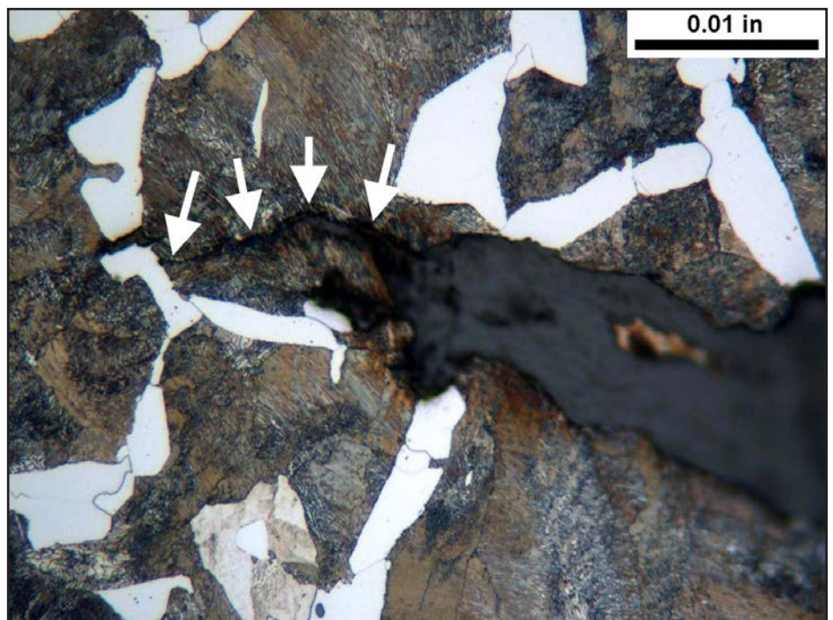
Figure 9 A higher magnification view of the right-center portion of Figure 8. Arrows indicate the presence of corrosion scale in tip of crack; 2% nital (OM 500×)
