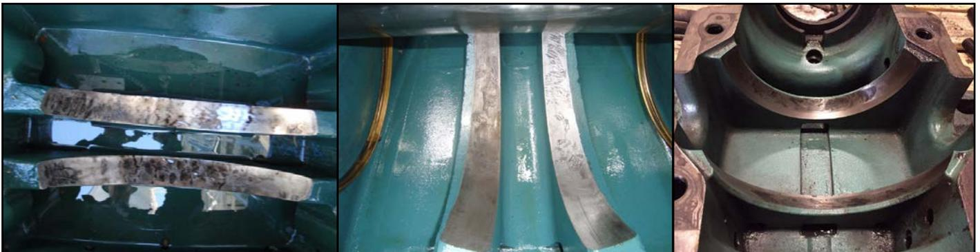
**Figure 4** Three separate housings that have been pulled from service due to high fan vibration levels and exhibit the characteristic fretting marks caused by improper contact and retention of the liner within the housing.
