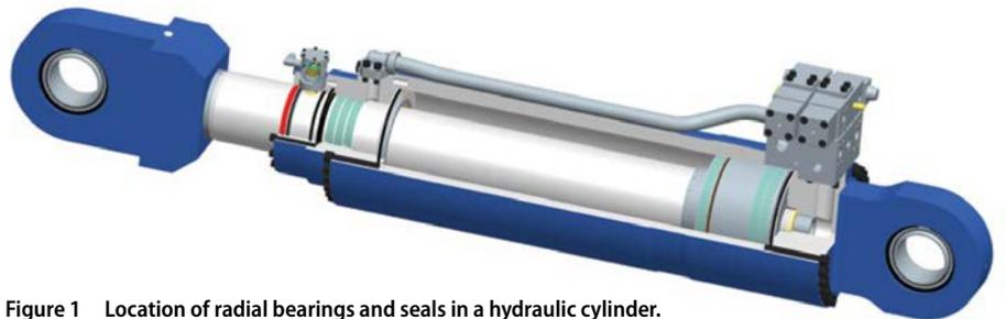
Figure 1 Location of radial bearings and seals in a hydraulic cylinder.
