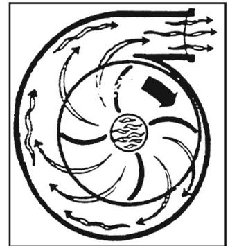
Figure 6 Centrifugal pump — variable torque load.
