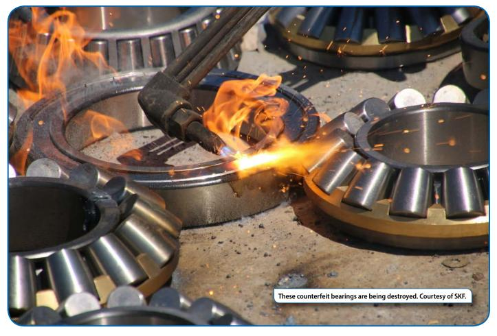
with counterfeit SKF bearings. Following just two days of operation, one of these bearings failed in a crucial application, forcing the costly, unplanned shutdown. After a complete analysis, SKF confirmed that the bearings were counterfeit. In cooperation with an SKF authorized distributor, the counterfeits were quickly replaced with genuine components.
