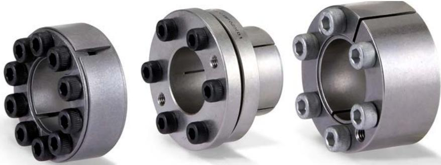
and easily. When tightened, these screws allow the inner and outer hub of the Posi-Lock to move along shaft contact surfaces. The movement between the inner and outer wedge of the Posi-Lock creates a tight, friction connection between hub, shaft and the Posi-Lock.
