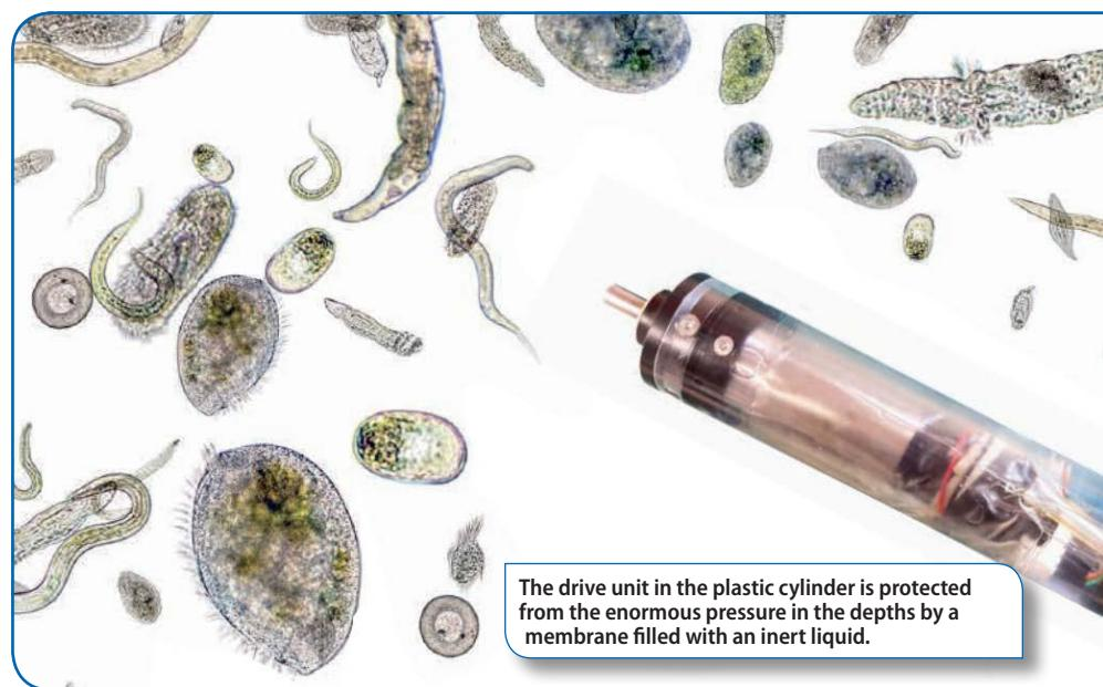
appropriate planetary gearheads. While some components are housed in a pressure stable titanium cylinder, some devices like the motors and gearboxes can only perform their work when in contact with the surroundings that are to be studied.
