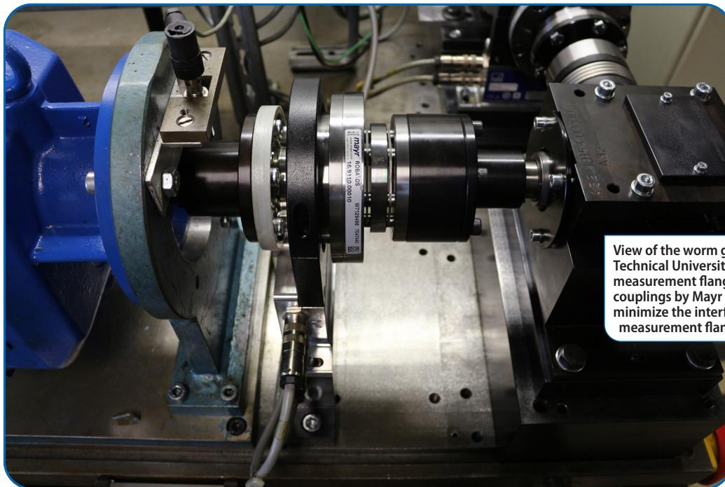
View of the worm gear test stand of the FZG at the Technical University of Munich: Together with the measurement flange, shaft misalignment compensation couplings by Mayr Power Transmission are used. They minimize the interference parameters affecting the measurement flange.
