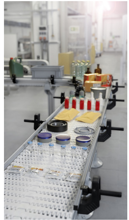
From electronics to consumer goods, VarioFlow plus fits multiple transport applications. (Photo: Bosch Rexroth)
