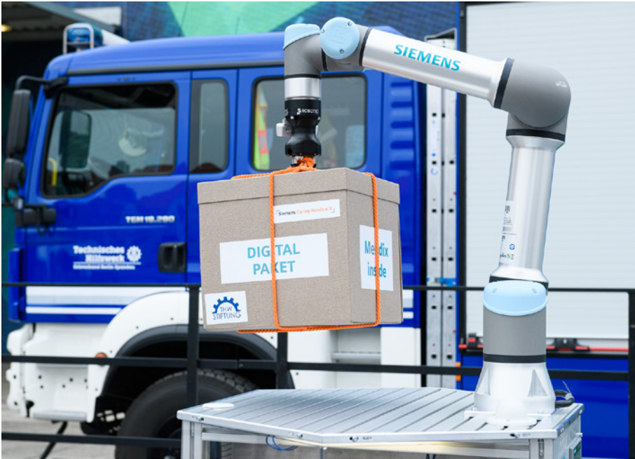
Robotics can stabilize throughput by performing repetitive tasks like pick-and-place, case packing, and palletizing with high precision and reliability. (Photo: Siemens)
