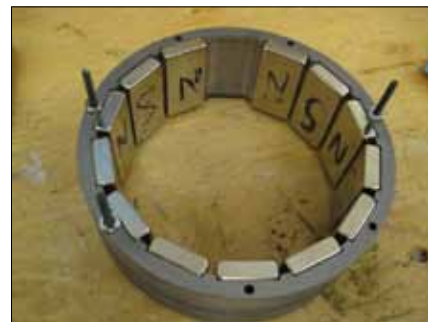
Figure 6—The rotor as it was fitted with magnets.
