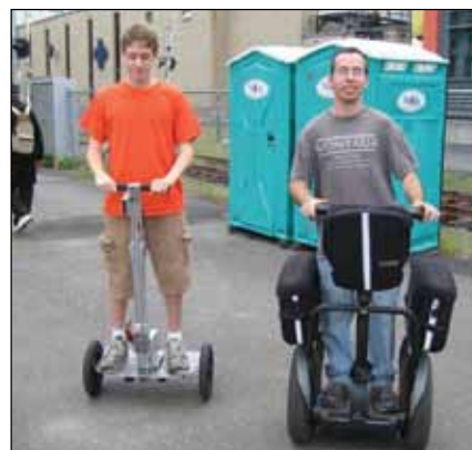
Figure 1—Our first project, a self-balancing electric scooter (left) built for under $1,000.
