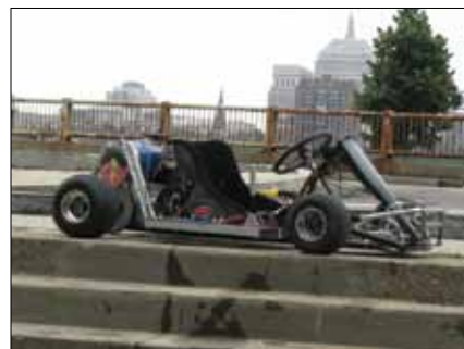
Figure 2—Our converted electric go-kart from 2008.
