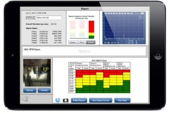
Tablet- and smartphone-based vibration analysis tools are speeding up response time to problems with rotating machinery (image courtesy of GTI Spindle Technology Inc.).
