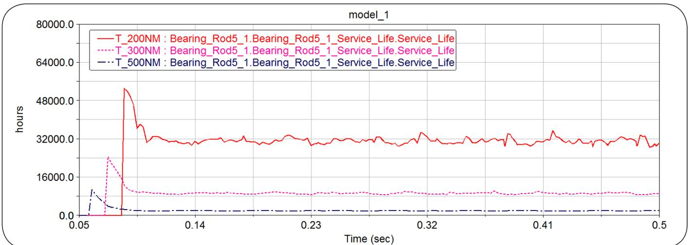
Figure 6 Bearing service life under different input torques.
