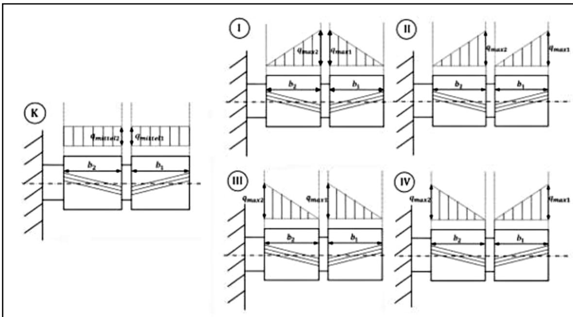
Figure 10 Adapted load cases for double helical gears.
