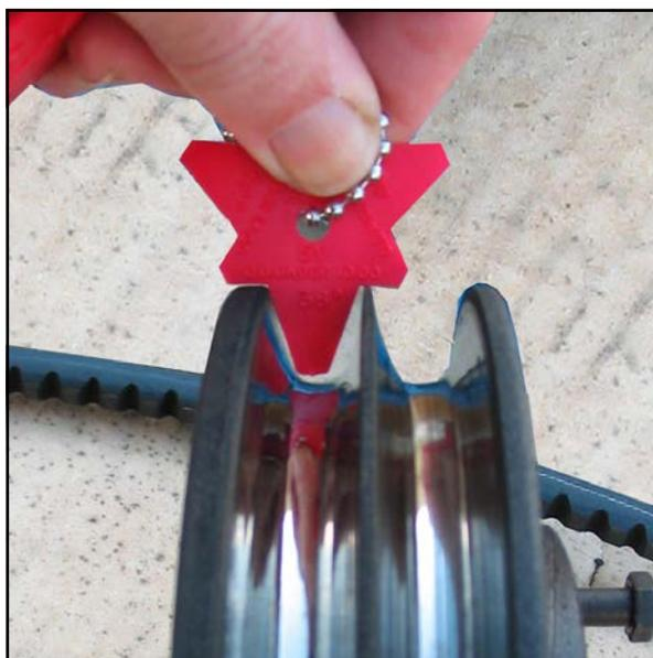
**Figure 10** This photo depicts a highly worn sheave, which can cause belt sidewalls to harden and crack, or produce excessive wear on the belt's bottom surface and corners, leading to premature belt failure. In an unworn sheave, the gauge should fit snugly into the groove with no light shining through.
