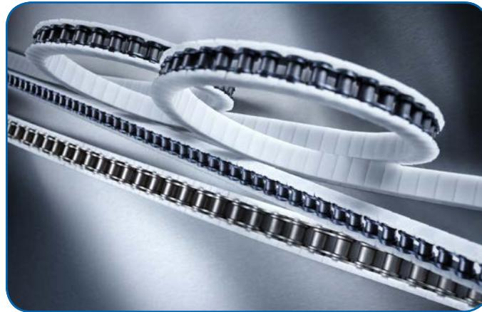
Iwis has developed a comprehensive range of transfer chains with durable plastic attachments to meet these requirements. The functional sections of the chain are completely enclosed, which offers a number of advantages: the product stays clean and undamaged, no dust or dirt can build up on the chain, goods are conveyed on a flat surface and there is no lifting of the load when the chain passes over the sprockets.
